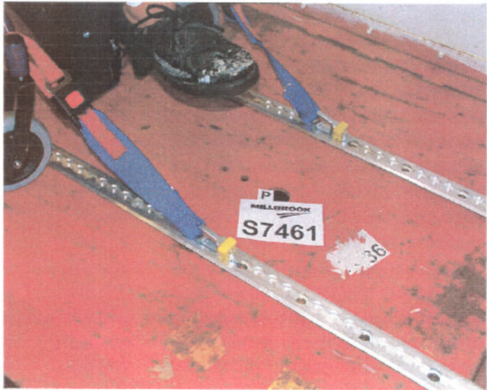
View of wheelchair front tie-downs, post-test
