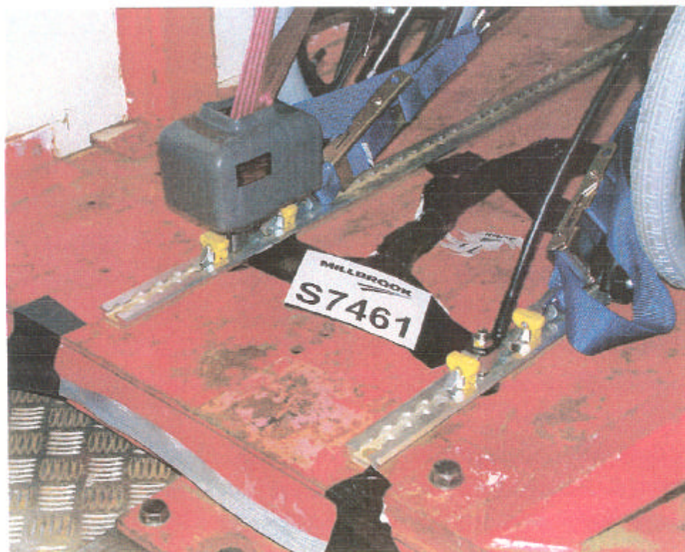
View of wheelchair rear tie-downs, pre-test
