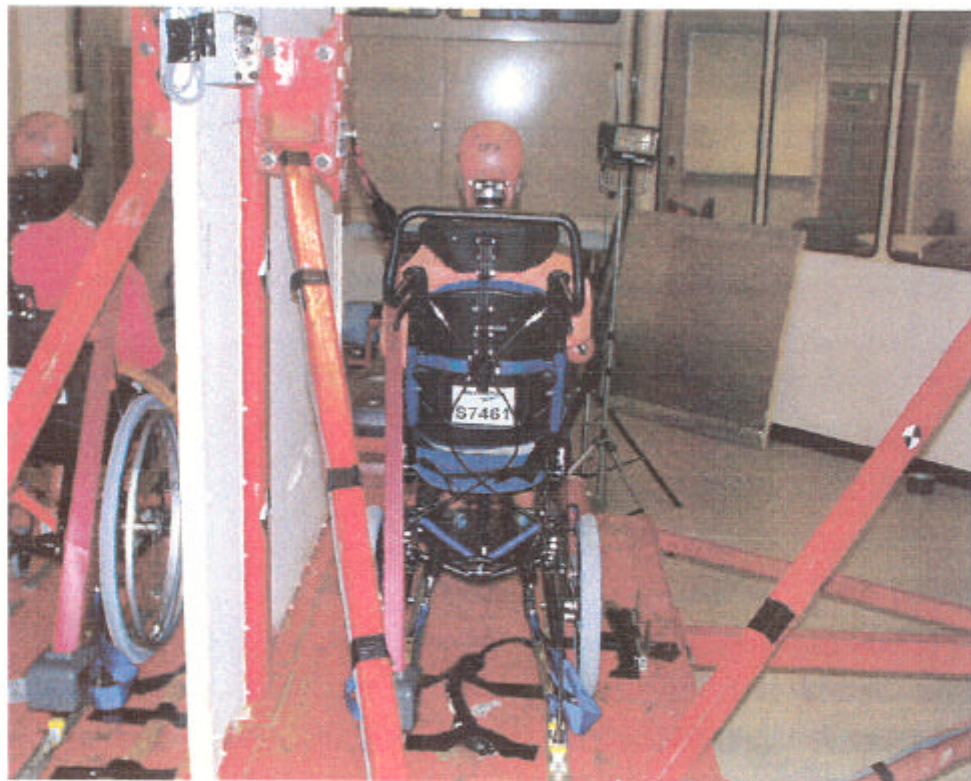
Rear view of wheelchair and occupant, pre-test
