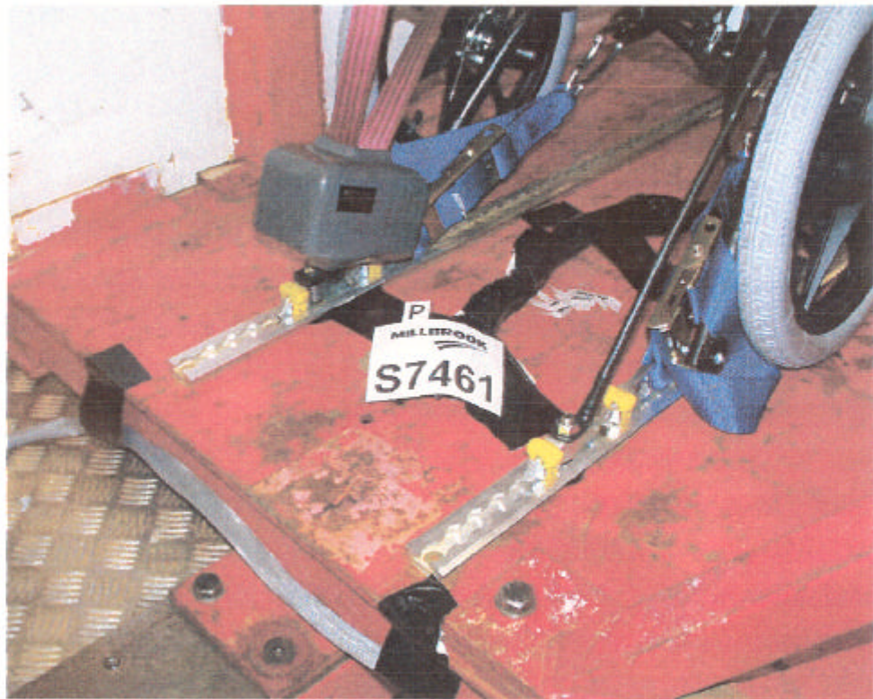
View of wheelchair rear tie-downs, post-test
