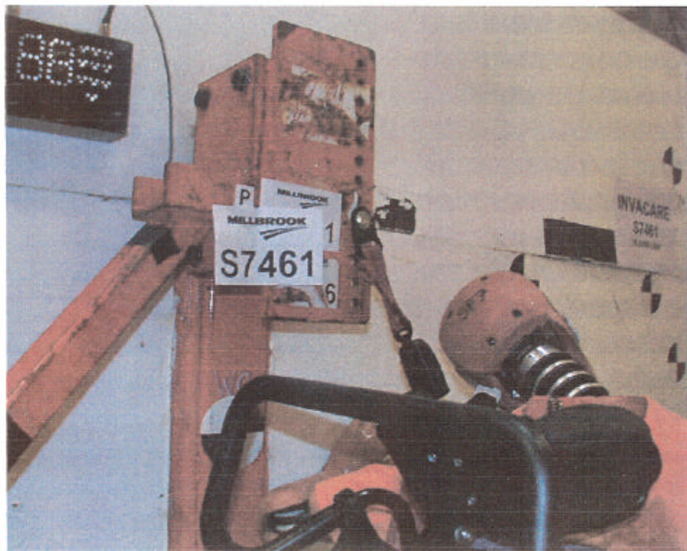
View of occupant upper torso anchorage, post-test
