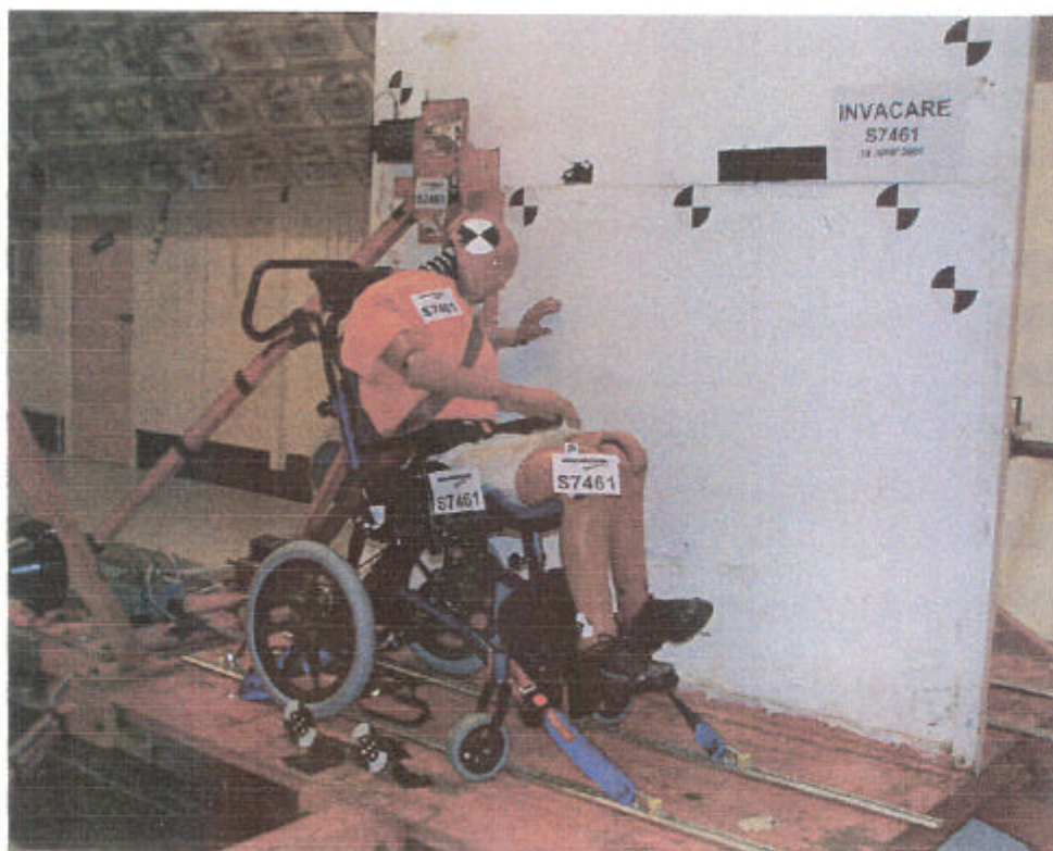
Front 3/4 view of wheelchair and occupant, post-test
