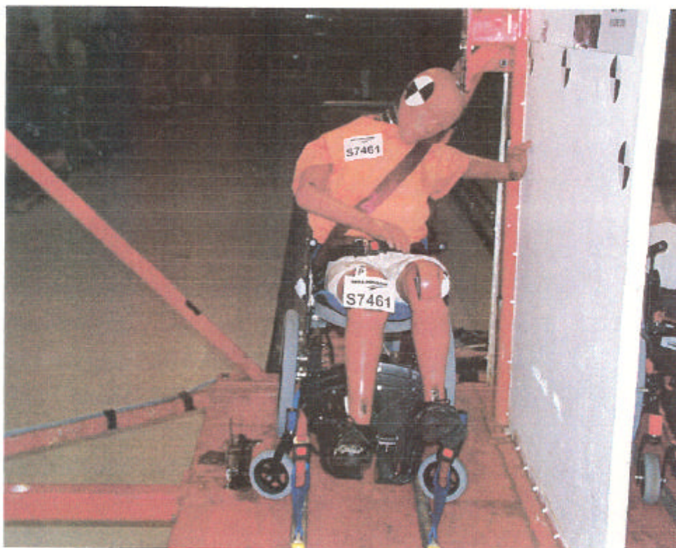
Front view of wheelchair and occupant, post-test
