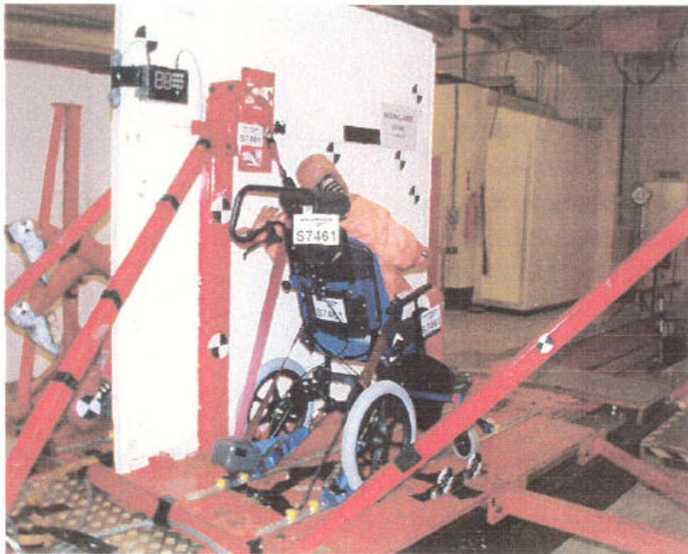
Rear 3/4 view of wheelchair and occupant, post-test
