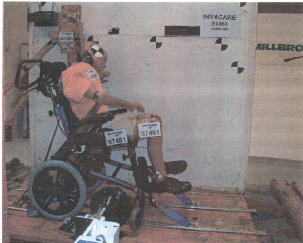
RH view of wheelchair and occupant, post-test
