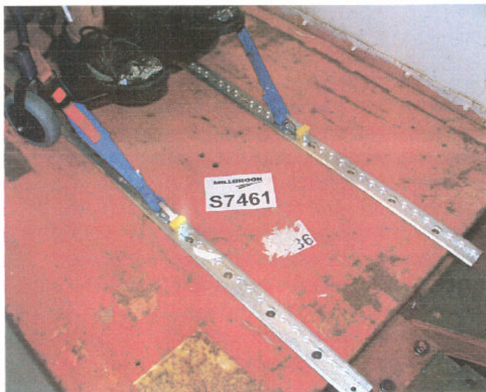
View of wheelchair front tie-downs, pre-test
