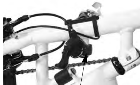
Force R and Force X parking brake with locking lever
