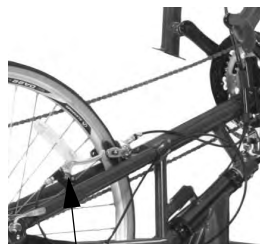
Force-2 parking brake with locking lever
