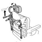
Loosen the handwheels  $\ensuremath{\boldsymbol{\triangle}}$  and raise the push handles as far as possible.
