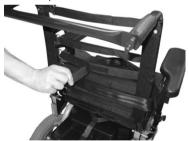
Adjust the tension of the individual straps as desired.
