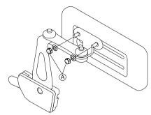
Loosen the two screws (A).
