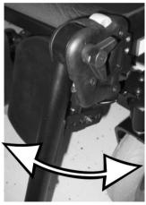
Move the legrest to the desired position. 10. Re-tighten the locking knob.
