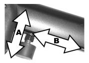
Move the rubber stop to the desired position.
