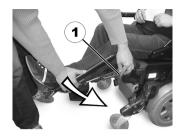
1. Keep the legrest in the foot plate area, pull the lateral adjusting lever (1) and lower the legrest slowly.
