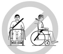
Seat belts may not be held at a distance from the user's body using parts of the mobility device such as armrests or wheels.
