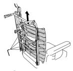
Loosen the screws  $\ensuremath{\mathbb{B}}$  and remove the backrest by lifting upwards.
