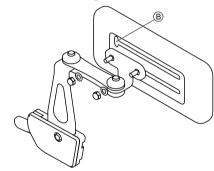
Remove hip pad bracket from mounting slot via cut-out (B).
