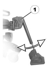
Loosen the screw (1) using the Allen key.
