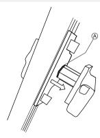
Depending on the side, the screw is accessible from the front or the rear.
