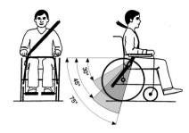
The pelvic belt should be positioned in the area between the user's pelvis and thighs so that it is unobstructed and not too loose. The ideal angle of the pelvic belt to the horizontal is between 45° and 75°. The maximum permissible angle is between 30° and 75°. The angle should never be less than 30°!
