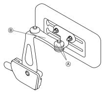
Remove upper screw and friction cap A.
