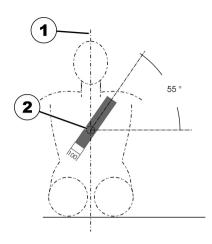
The safety belt installed in the transporting vehicle should be applied as shown in the illustration above.
