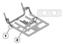
On both sides, remove the screws, washers, and cover plates (1).
