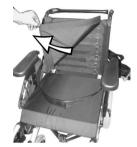
Remove the backrest cushion (attached with hook–and–loop straps) by pulling it up and off to access the adjustment straps.
