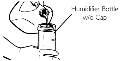
FIGURE 6.3 Filling the Humidifier
