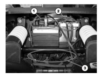
• Pull the motor plug (3) out of the electronic module.
