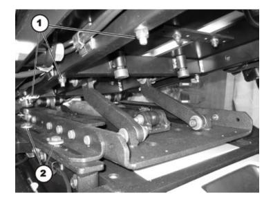
• Undo the six nuts (1) with a 13/32" socket spanner and remove the six 5/32" Allen screws.
