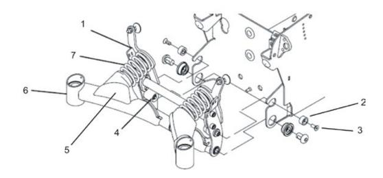
• Ensure that the rear springs (7) are compressed:
