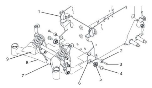
• Position the complete rear wheel suspension between the two mounting points (6).
