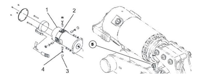
• Disengage the motor (1) by setting the engaging lever to "Push".
