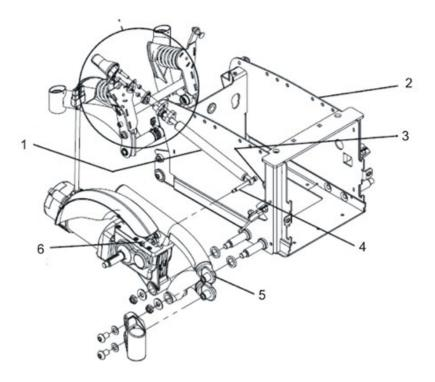
• Push the gas cylinder (1) from the front towards the rear into the holder until the bottom end is just in front of the hole (3) in the battery case (2) and you can insert the screw (4).
