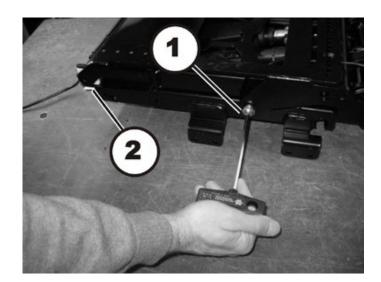
• Undo and remove the seat support Allen screws (1) on the left-hand and right-hand side of the mobility device.
