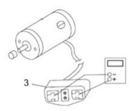
• Connect the digital multimeter to the motor plug contacts (3) and measure the resistance between the contacts.
