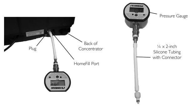
FIGURE 25.5 Pressure Testing
