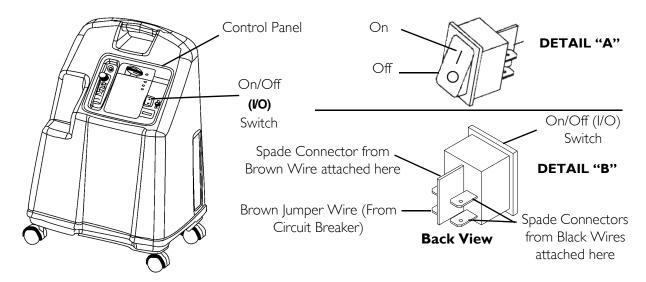
FIGURE 17.1 Replacing On/Off Switch
