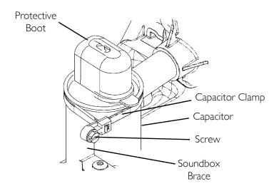
FIGURE 7.4 Replacing Capacitor
