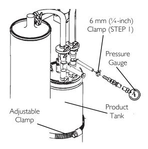
FIGURE 25.3 Pressure Testing
