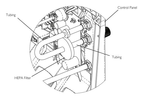
FIGURE 6.3 Replace the Outlet HEPA Filter after 06/09/06
