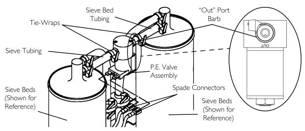
FIGURE 8.1 Replacing P.E. Valve
