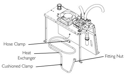
FIGURE 12.1 Replacing Heat Exchanger - Platinum 5 Models Manufactured Before 9/9/2005
