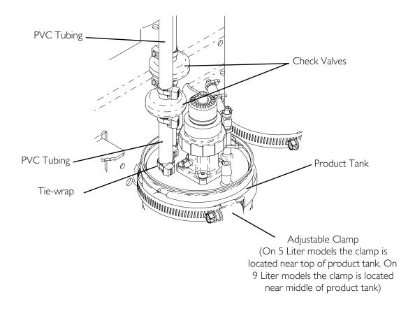
FIGURE 10.1 Replacing Check Valves
