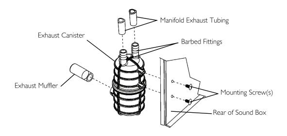
**FIGURE 6.5** Replacing Exhaust Canister/Exhaust Muffler (Platinum 5 Manufactured before 7/24/03)
