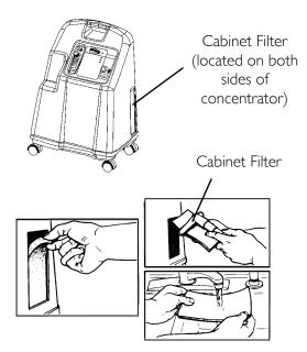
FIGURE 6.1 Cleaning the Cabinet Filter
