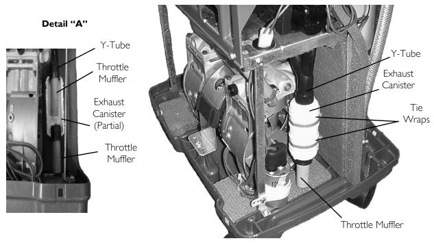
FIGURE 6.7 Inspecting/Replacing the Throttle Muffler (Platinum 5 and 9 AWQ)
