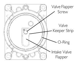
FIGURE 7.7 Removing Compressor and Compressor Heads - Rebuilding the Compressor - O-ring, Intake Valve Keeper and Valve Keeper Strip
