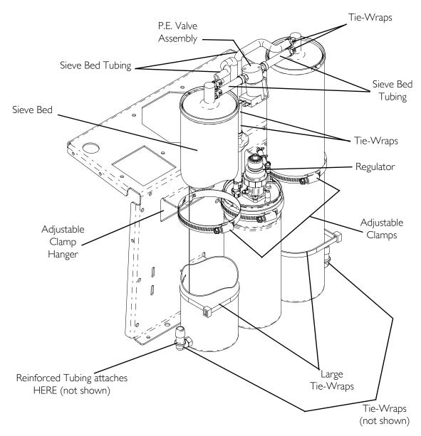
FIGURE 9.1 Replacing Sieve Beds - 5 Liter models manufactured before 1/27/05
