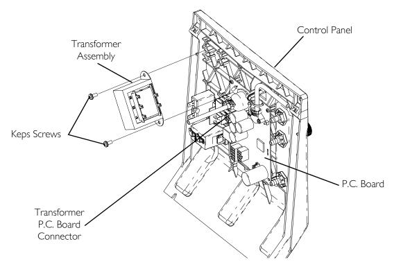
FIGURE 16.1 Replacing Transformer Assembly
