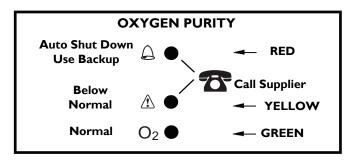
FIGURE 21.1 Indicator Light Explanation (SensO<sub>2</sub> Models)
