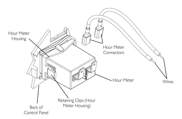
FIGURE 19.1 Replacing Hour Meter
