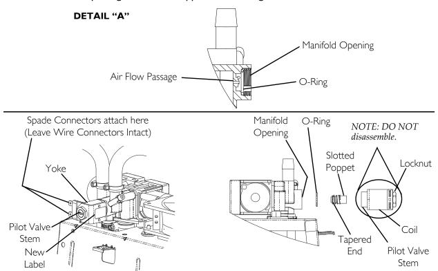
**FIGURE 20.6** Replacing Pilot Valve Poppets and O-Rings - 5 Liter Manufactured After 8/1/05 and 9 Liter models
