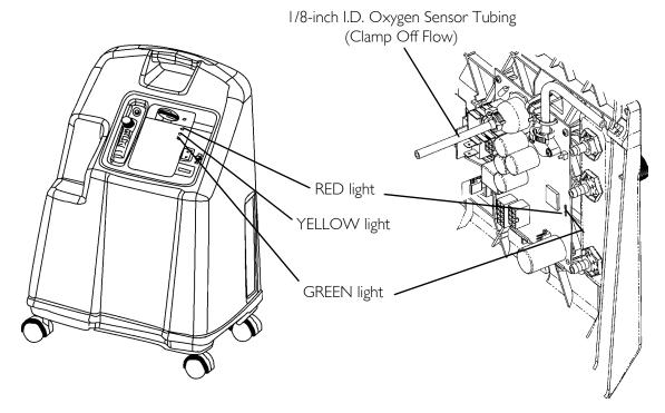
FIGURE 24.3 Oxygen Sensor
