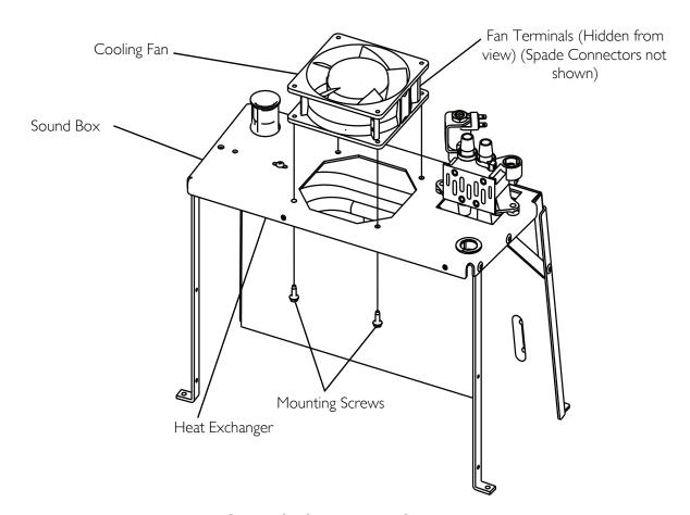
FIGURE 14.1 Replacing Cooling Fan
