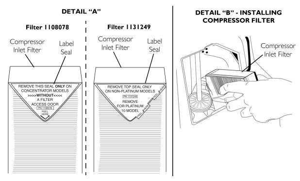
FIGURE 6.4 Replacing the Compressor Inlet Filter
