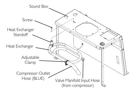
FIGURE 12.3 Replacing Heat Exchanger
