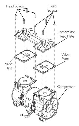
FIGURE 7.5 Removing Compressor and Compressor Heads - Rebuilding the Compressor - Compressor - Compressor Head Plate - Valve Plates
