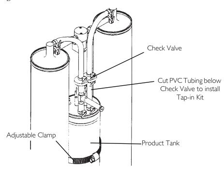
FIGURE 25.1 Disassembly
