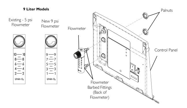
FIGURE 18.1 Replacing Flowmeter
