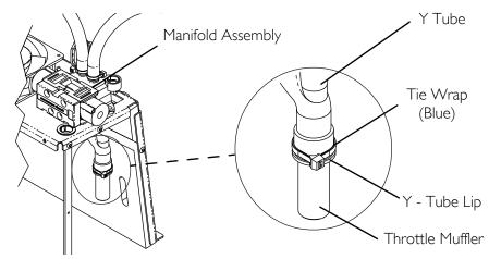
**FIGURE 6.6** Inspecting/Replacing Throttling Muffler (Platinum 5 AW Manufactured after 7/24/03)
