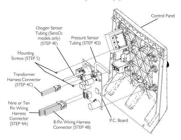
FIGURE 15.1 Replacing P.C. Board
