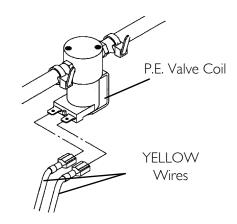
FIGURE 24.4 P.E. Valve Coil Test
