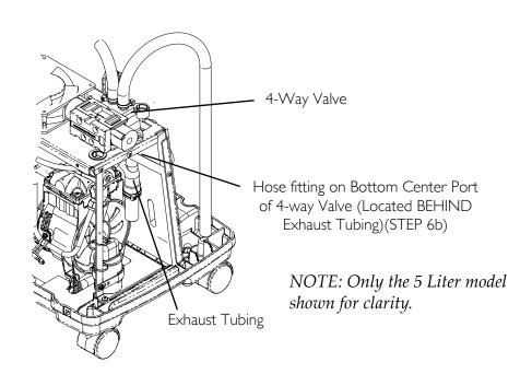
FIGURE 23.1 Leak Test
