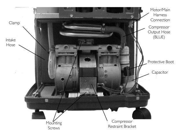
**FIGURE 7.3** Replacing Compressor Assembly - 9 Liter Models
