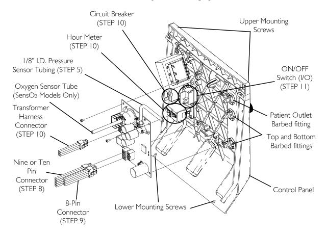
FIGURE 13.1 Removing Control Panel
