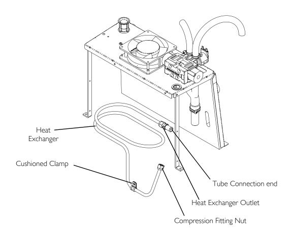
FIGURE 12.2 Replacing Heat Exchanger - Platinum 5 Models Manufactured After 9/9/2005
