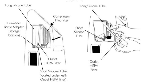
FIGURE 6.2 Replace the Outlet HEPA Filter before 06/09/06
