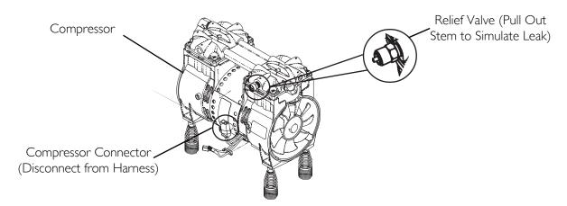
FIGURE 24.1 Low Pressure Test - Time-Out Test
