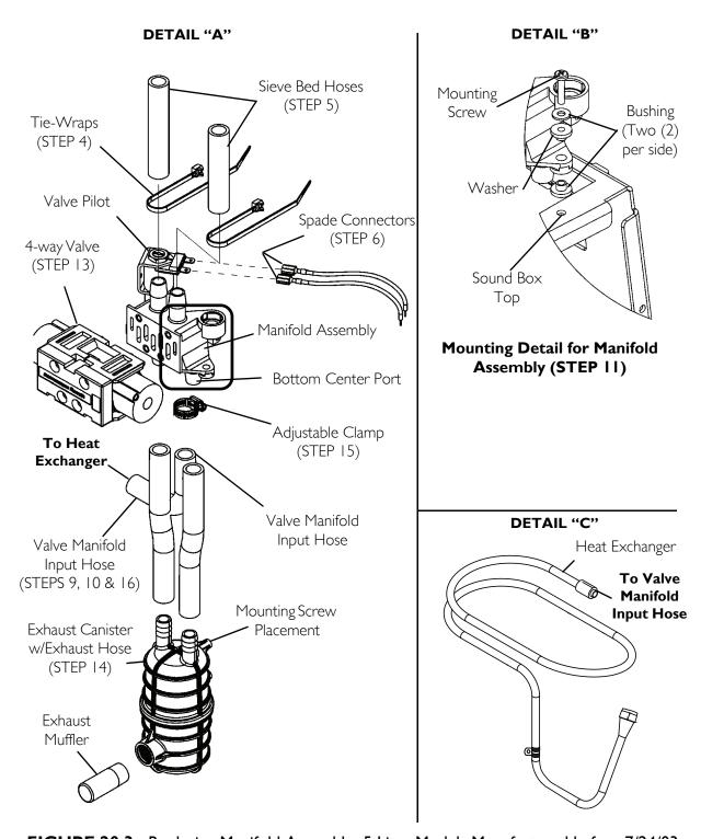
FIGURE 20.3 Replacing Manifold Assembly- 5 Liter Models Manufactured before 7/24/03
