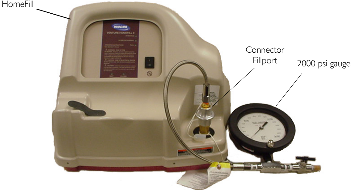
FIGURE I4.3 HomeFill 2000 psi Switch/P.C.B. Shut Down Test
