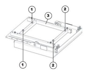
The picture shows the seat frame with the drillholes for the standard seat.
