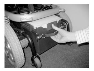
Pull the battery cases out using the side handles.
