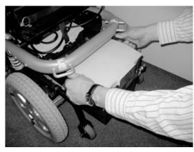
Pull the front battery case backwards using the belt and pull it out using the handles.
