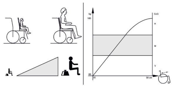
For best possible driving characteristics of rear-wheel drive wheelchairs, the weight to be distributed: 30 - 40 % front and 60 - 70 % rear.
