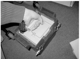
Remove the terminal cover from the battery terminals (1).
