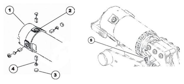
Disengage the motor (1) by setting the engaging lever to "Push".
