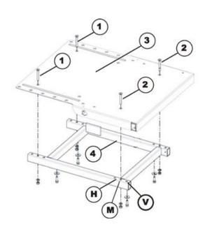
The picture shows where the drillholes for fixing the seat frame (3) are located on the base frame.
