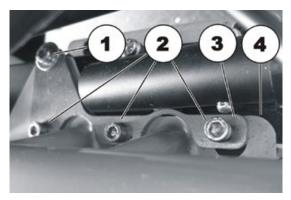
A further reinforcing plate (1) is located under the splash guard.
