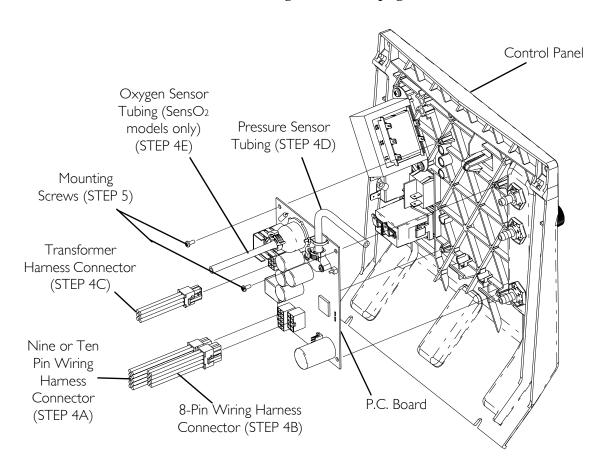
FIGURE 15.1 Replacing P.C. Board
