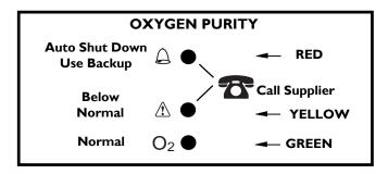
FIGURE 21.1 Indicator Light Explanation (SensO2 Models)
