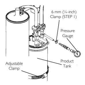
FIGURE 25.3 Pressure Testing
