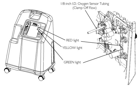
FIGURE 24.3 Oxygen Sensor
