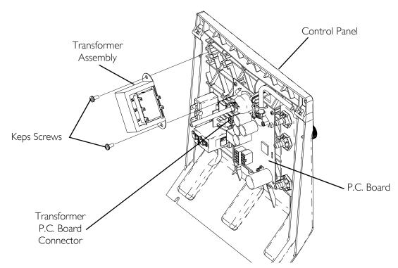
FIGURE 16.1 Replacing Transformer Assembly
