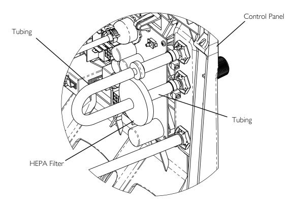
FIGURE 6.3 Replace the Outlet HEPA Filter
