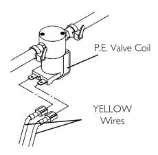
FIGURE 24.4 P.E. Valve Coil Test
