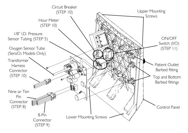
FIGURE 13.1 Removing Control Panel
