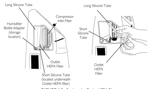
FIGURE 6.2 Replace the Outlet HEPA Filter
