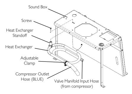
FIGURE 12.4 Replacing Heat Exchanger
