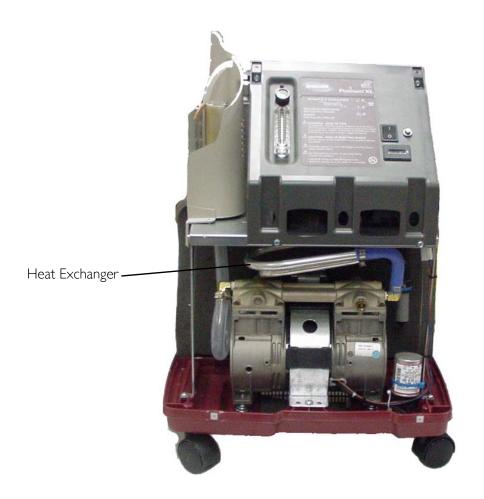
FIGURE 6.8 Cleaning the Heat Exchanger
