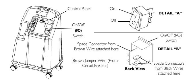
FIGURE 17.1 Replacing On/Off Switch
