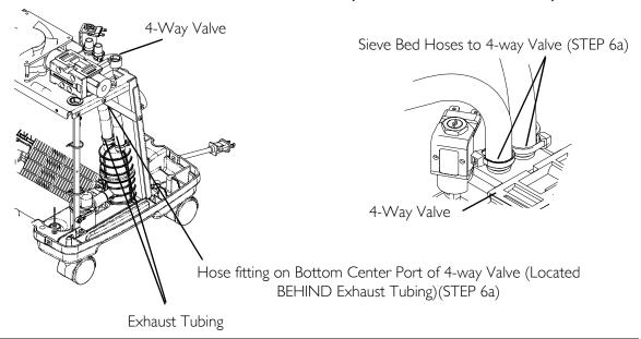
For 5 Liter Models with Throttle Muffler (manufactured after 7/24/03) and 9 Liter Models
