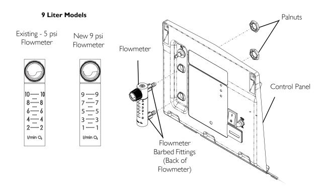
FIGURE 18.1 Replacing Flowmeter
