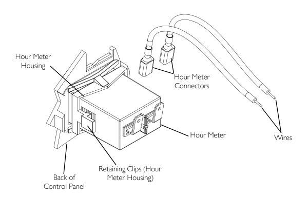
FIGURE 19.1 Replacing Hour Meter
