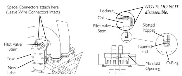
FIGURE 20.5 Replacing Pilot Valve Poppets and O-Rings - 5 Liter Manufactured Before 8/1/05
