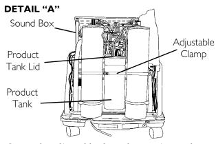
*NOTE:* The adjustable clamp hanger is not shown. It is located behind the product tank and is attached NOTE: Sieve Beds removed for clarity. to the sound box.
