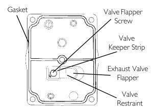
FIGURE 7.8 Removing Compressor and Compressor Heads - Rebuilding the Compressor - Exhaust Valve Flapper, Valve Restraint and Valve Keeper Strip
