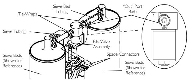
FIGURE 8.1 Replacing P.E. Valve
