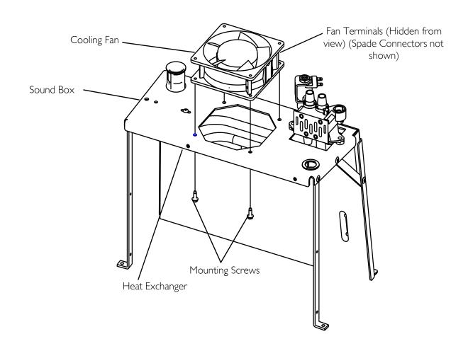
FIGURE 14.1 Replacing Cooling Fan
