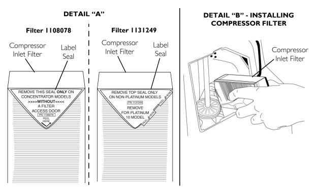
FIGURE 6.4 Replacing the Compressor Inlet Filter
