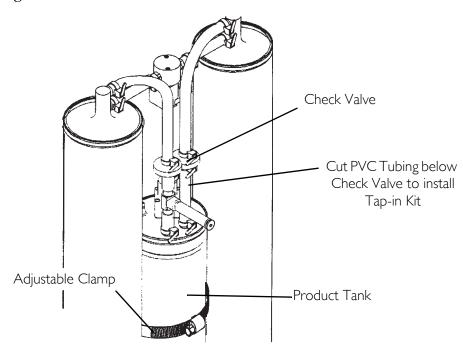
FIGURE 25.1 Disassembly
