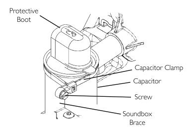
FIGURE 7.4 Replacing Capacitor
