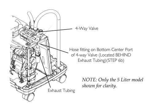
FIGURE 23.1 Leak Test
