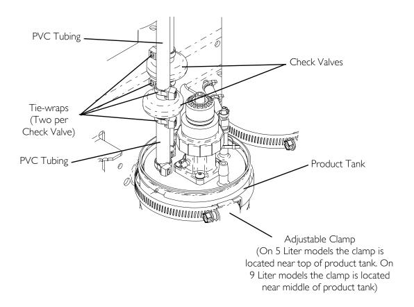
FIGURE 10.1 Replacing Check Valves
