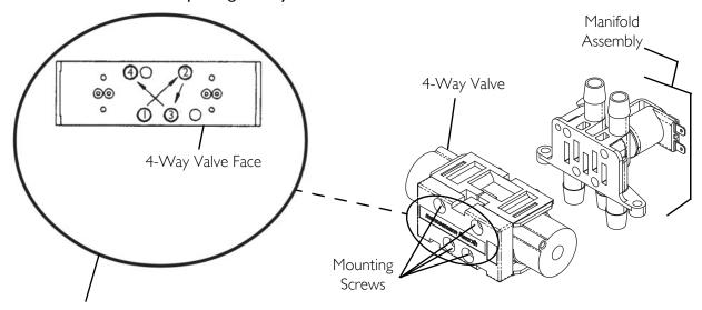
*NOTE: The Numbers indicate the mounting screw torque sequence: pre-torque to* 1.1 N-M  $\pm$  0.2 N-M (10 in-lbs  $\pm$  2 in-lbs), then *torque to* 2.5 N-M  $\pm$  0.2 N-M (22 in-lbs  $\pm$  2 in-lbs).
