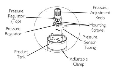
FIGURE 11.1 Replacing/Adjusting Regulator
