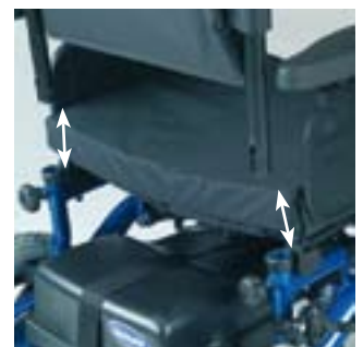
The back comes off simply by loosening the two hand wheels at the back.
