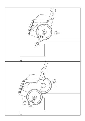
While descending stairs always push the scalamobil slightly forward, away from you, until the brakes grip on the edge of the following step. Also the scalamobil needs to remain tilted approximately in the same angle. Finally, never release the grips of the scalamobil!
