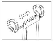
Push handle into the desired position (locking device automatically reengages).
