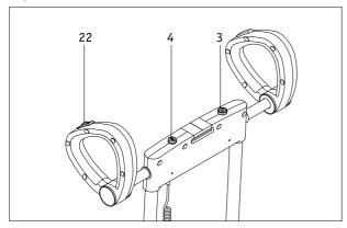
The scalamobil is switched on or off by pressing the On/Off button [3]. When switching on the display element [4] simultaneously shows the last direction of travel selected on the direction of travel switch [22] and the state of charge of the battery.
