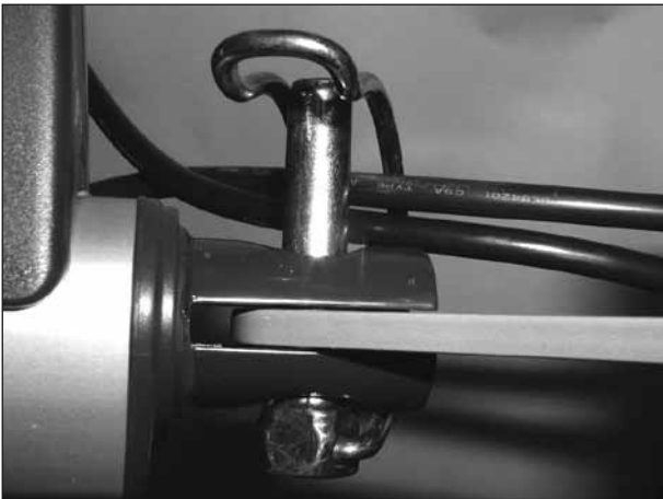
Wiring of the leg section motor and bed end motor (foot) through the backrest motor pipe pin.
