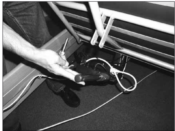
2) Remove the pipe pin from the backrest motor.
