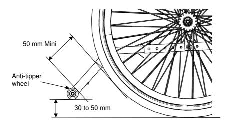
FIGURE 9.3 Adjusting Anti-Tippers
