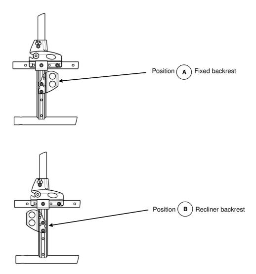
FIGURE 5.6 Possible Positions of Wheel Plate
