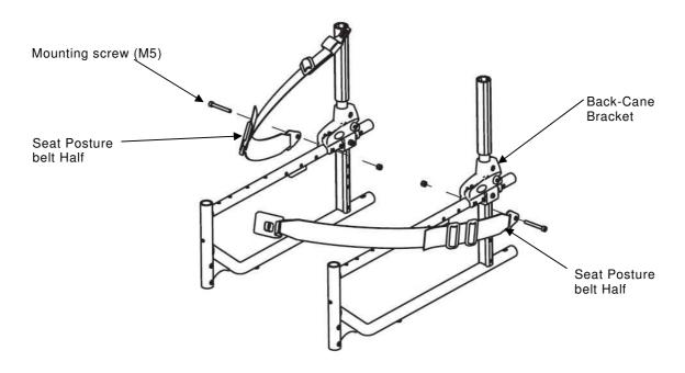
FIGURE 4.11 Installing/Removing Seat Posture Belt
