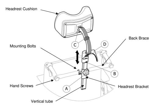
FIGURE 8.2 Installing Headrest
