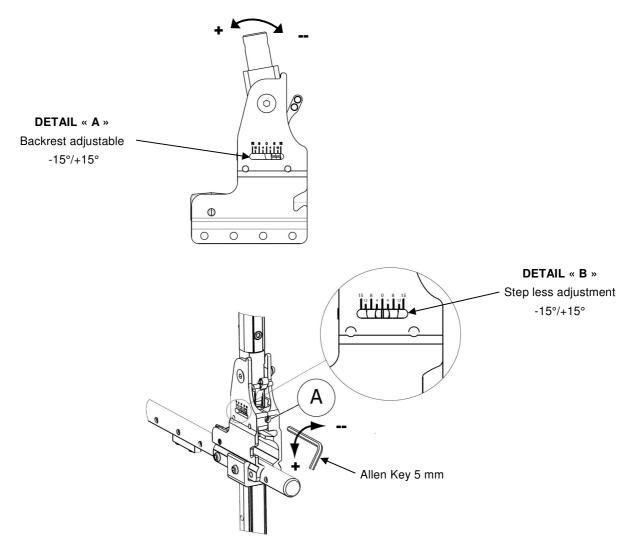
FIGURE 4.6 Adjusting the Angle Adjustable Backrest
