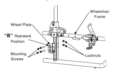
FIGURE 5.5 Adjusting the Wheelbase Length
