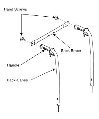
FIGURE 4.12 Installing/Removing the Standard Back brace
