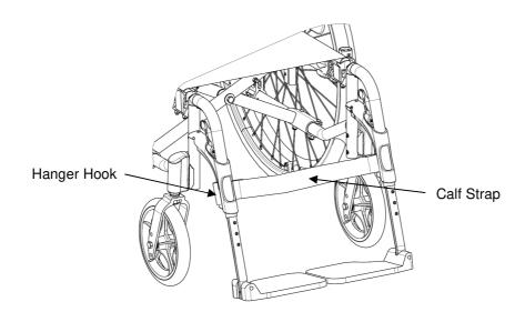
FIGURE 2.3 Installing Calf Strap
