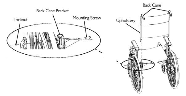
FIGURE 4.1 Removing Standard Back-Canes
