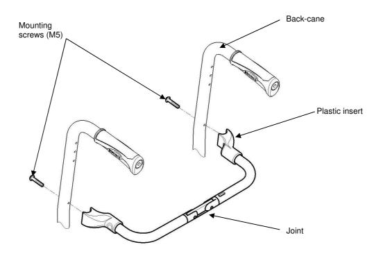
FIGURE 4.13 Installing/Removing the Folding Back Brace
