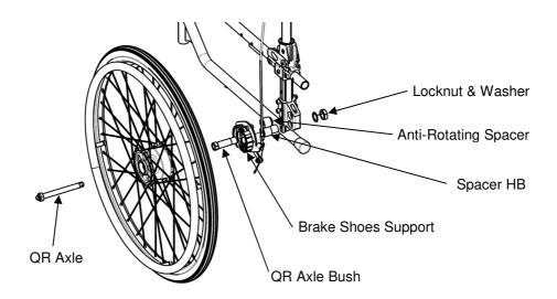
FIGURE 7.4 Installing Hub Brakes
