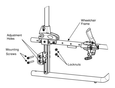
FIGURE 5.7 Adjusting Rear Wheel Height
