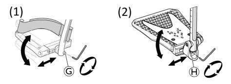
FIGURE 2.4 Installing Angle Adjustable Footplate
