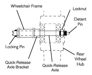
FIGURE 5.3 Adjusting Quick-Release Axles
