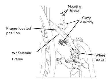
FIGURE 7.1 Adjusting Wheel Brakes - Adjusting Wheel Brake Position
