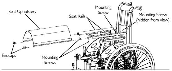
FIGURE 4.2 Removing/Installing Seat Upholstery
