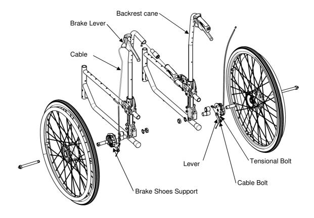
FIGURE 7.5 Installing/Adjusting Hub Brake
