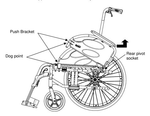
FIGURE 3.2 Removing/Installing Swing Away Armrest
