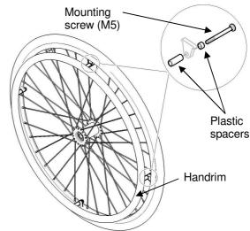
FIGURE 5.4 Replacing Handrims
