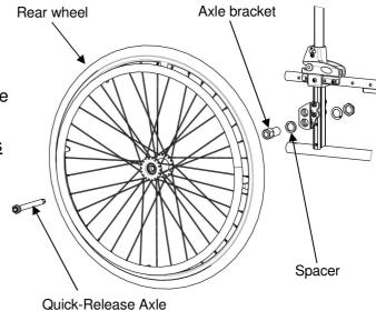
FIGURE 5.2 Removing/Installing Rear Wheels
