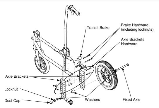
FIGURE 5.1 Removing/Installing Rear Wheels
