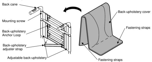
**FIGURE 4.4** Installing/Replacing Contour (adjustable) Back Upholstery
