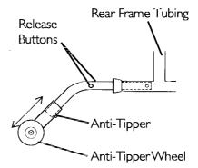
FIGURE 9.1 Installing Simple Anti-Tippers
