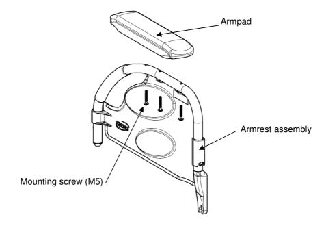
FIGURE 3.3 Replacing Armrest Arm Pad
