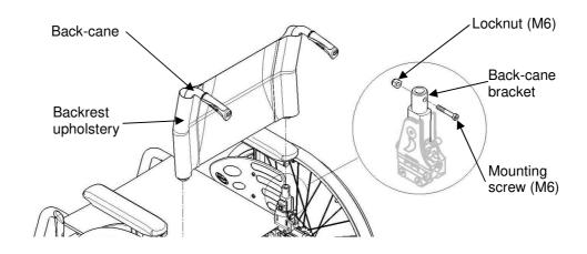
FIGURE 4.1 B Removing Angle Adjustable Back-Canes
