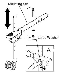
FIGURE 9.2 Installing Anti-Tippers with Tipping Aid
