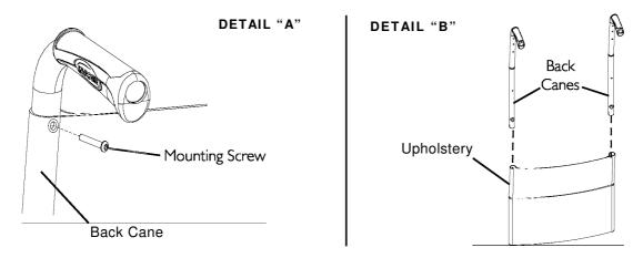
FIGURE 4.3 Removing/Installing Standard Back Upholstery
