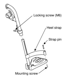
FIGURE 2.2 Replacing Heel Strap
