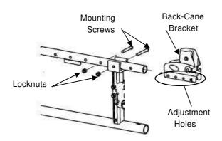
FIGURE 4.10 Removing/Installing/Adjusting the Back-Cane Bracket
