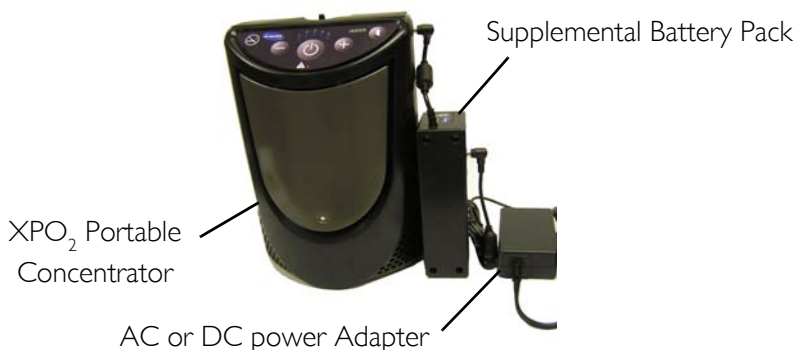
FIGURE 6.5 Charging the Internal and Supplemental Battery Pack Simultaneously
