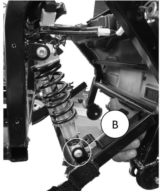
Loosen and remove lower bolt (B) on rear shock absorber on left and right side of mobility device.
