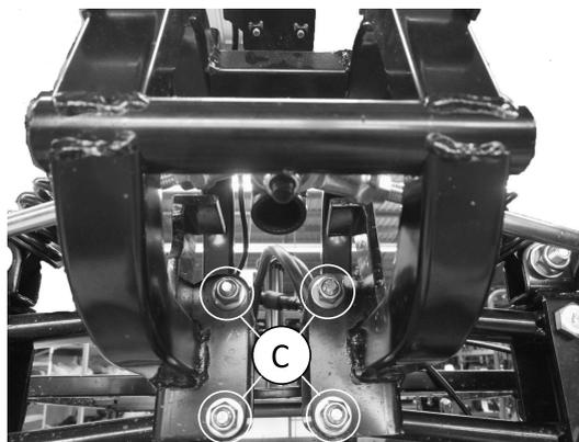
Loosen four screws **C** that fix cross members to frame.
