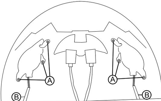
Remove direction indicator screw (A) on housing.
