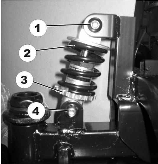
1. Remove top screw (1) on shock absorber (2).
