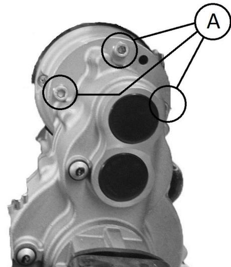
Loosen three Allen screws (A).
