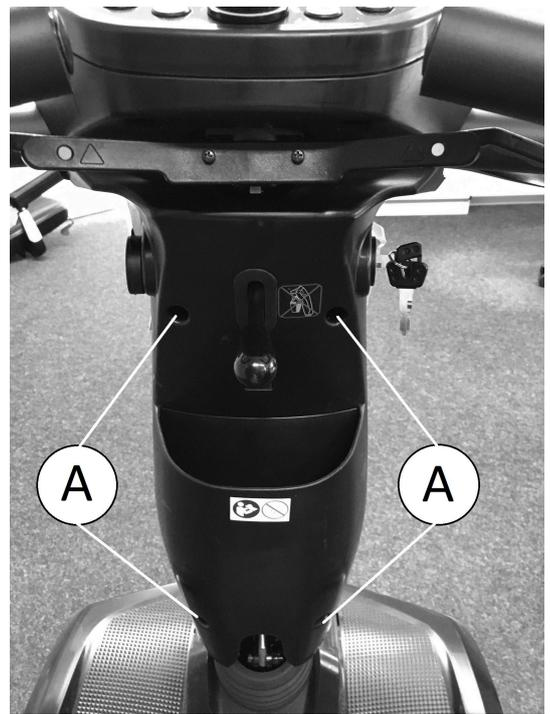
5. Remove screws **A** on rear steering column shroud.
