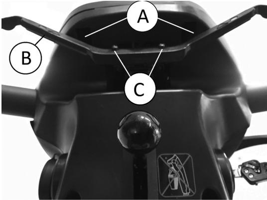
Remove screws (A) below operating console.
