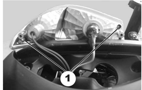
Remove screws (1) on rear light glass.
