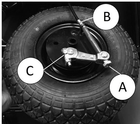
Slacken brake cable using setting screw **A**.
