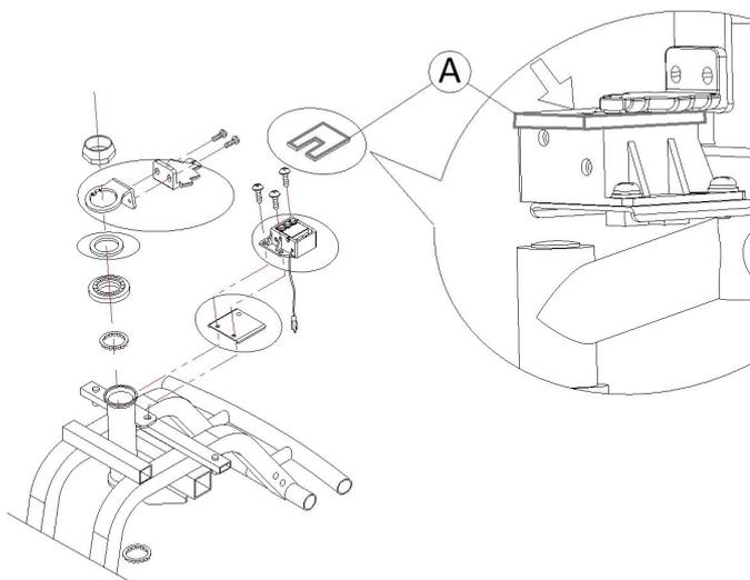
To check position of sensors of curve control device, use measuring gauge (A) supplied in "Bend speed reducer retrofitting kit".
