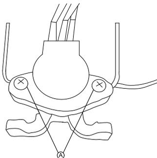
Remove screws (A) on potentiometer.
