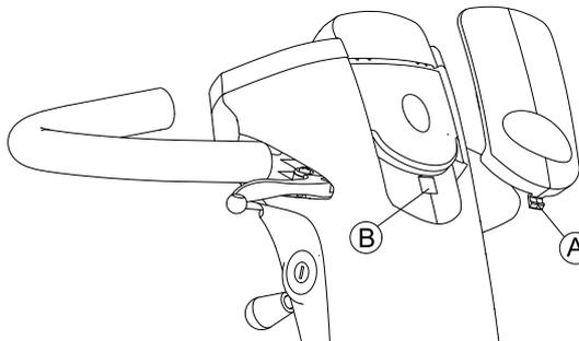
Remove top shroud **A** from steering column **B**.
