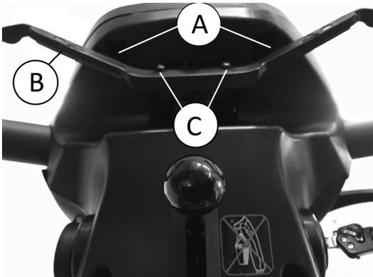
1. Remove drive lever screws **C**.
