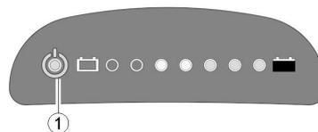
**i** The ON/OFF diode (1) is used as a fault display (status display). It will flash if there is a problem with the scooter. The number of flashes indicates the type of error. Refer to 4.2.3 Error codes and diagnostic codes, page 8.
