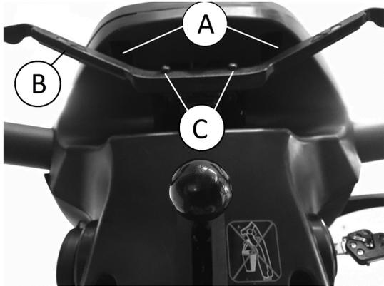
Remove screws (A) below operating console.
