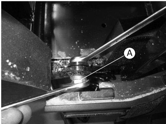
Loosen and remove screw (A) that attaches swing arm to chassis on left and right side of the mobility device.
