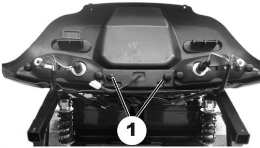
Remove screws (1) on brake light.
