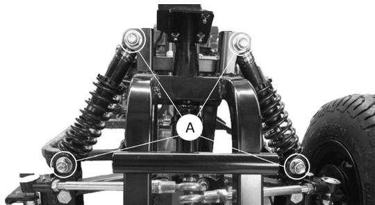
Loosen 4 screws **A** on front shock absorbers.
