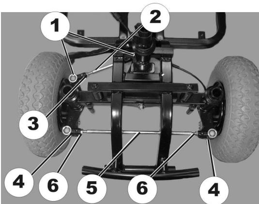
2. Remove circlip (1) on steering link (2).
