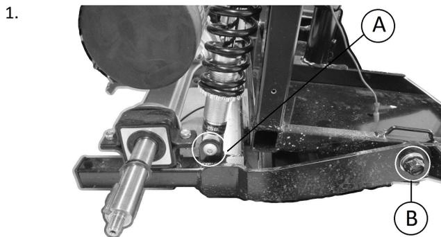
1. Loosen and remove screw **B** on swing arm. For replacing swing arm, see 4.8.3 Replacing swing arm, page 22 .
