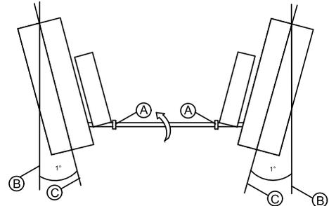
Spin steering link up by 0,5 cm. Wheels stand turned inwards by 1° (C) from neutral position (B).
