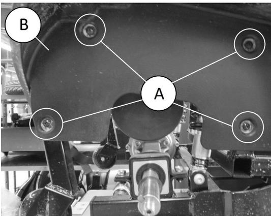
Remove screws (A) on mud guard.
