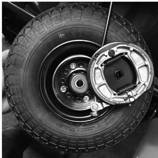
Pull brake out of brake drum.
