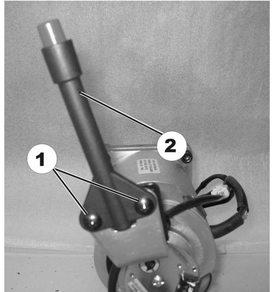
Remove screws (1) on disengaging lever (2).
