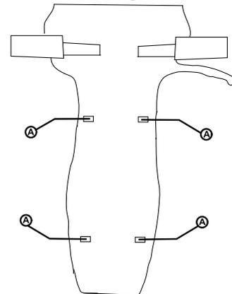
11. Remove screws **A** on front steering column shroud.
