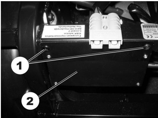
Remove both screws (1) from lifter controls (2).
