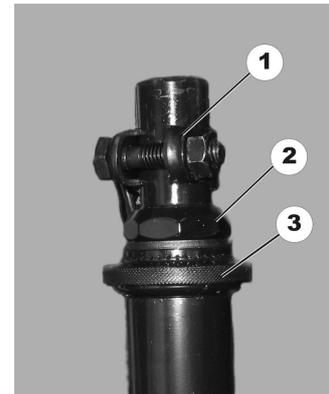
14. Loosen and remove screw at clamp (1).
