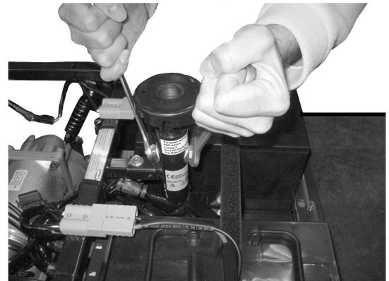
Remove securing bolt, nut and washers of seat support tube.
