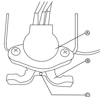
Connect potentiometer (A) and drive lever mounting (B):
