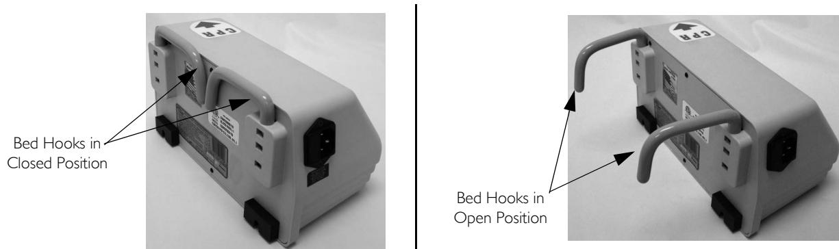
FIGURE 2 Installing the Power Unit
