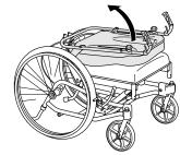
Unfold the backrest into an upright position.
