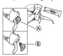
The locking device A allows you to set the tilting of the seat unit and/or the angling of the backrest to a fixed position.
