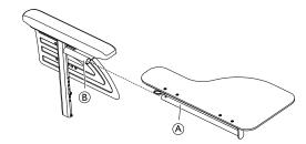
Insert the tube of the half tray (A) into the attachment
