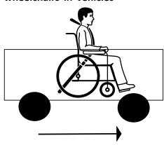
The wheelchair and user should be transported forward-facing in the travel direction. All auxiliary equipment such as tables, trunk support, abduction cushion etc should be removed and stored safely so that they do not injure anyone during any kind of accident.
