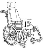
Push the footrest down into the tubes of the legrest attachment.
