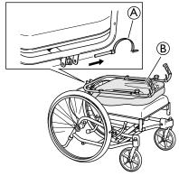
Remove the safety pin (A) and fold the backrest (B).
