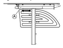
1. Slide the half tray (A) forwards or backwards to adjust to the required depth.
