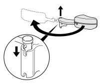
The "swing-away" trunk support can be turned sidewards in order to be out of the way when the user is moving in to or out of the wheelchair.
