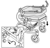
Remove the pin  ${\Bbb C}$  from the lower gas piston  ${\Bbb D}$  to reduce the height of the folded chair even more.
