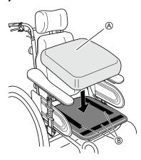
The seat depth of the chair can easily be adjusted to provide good support. The width between the legrests and armrests and the height of the armrests can also be adjusted.
