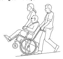
$\mathring{\parallel}$  The wheelchair can manage a slope of 15°.
