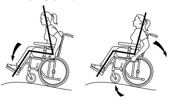
Many experienced users can propel themselves up a slope. In order not to lose control of the steering and to avoid tipping backwards, you should always lean forwards whilst propelling up a slope. Propel the wheelchair forwards using short, quick strokes applied to the hand rims, in order to maintain speed and steering control.
