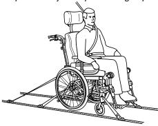
The wheelchair should be secured in the vehicle with a 4-point restraint system. The user should wear a 3-point safety belt secured in the vehicle.
