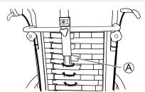
Adjust the shape of the "Laguna" tension adjustable backrest with the velcro® straps
