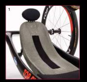
1. The totally adjustable featherweight carbon fiber back is as lightweight as the fixed welded back, allowing athletes the ability to find their most aerodynamic and powerful position for the course, whether it is a road race, time trial or triathlon.
