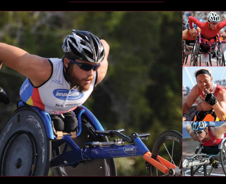
The **Invacare® Top End® Eliminator™ OSR Racing Wheelchair** is designed for speed. The super-stiff roll-formed horizontal maintube, combined with a relaxed headtube angle for exceptional stability and aerodynamics, make it the choice of champion racers like Ernst van Dyk, Krige Schabort, Kurt Fearnley, Chantal Petitclerc and Edith Hunkeler. So, if you have your sights set on winning, the Eliminator OSR racing wheelchair will help you get to the finish line first.
