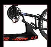
5. The redesigned curved monocoque front triangle is super strong and looks terrific. This new design allows the athlete to get closer to the front wheel which translates to a lighter and stiffer fork because it is shorter. Plus, it allows for more body clearance so the athlete can get lower and obtain a more streamlined position.
