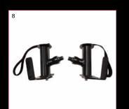
8. The quad cuff power plate handpedals feature an adjustable quad cuff to accommodate various hand sizes and positions. There is a detachable strap that fastens to the quad cuff if needed. The lower power plate will help you power through your stroke on the downstroke and the upper power plate will do the same on the upstroke. Most athletes customize their handpedals once they start riding by adding bicycle handlebar tape to optimize their pedal power.
