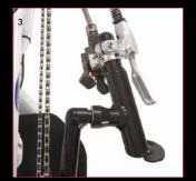
3. The SRAM<sup>®</sup> X9 30 speed drive train, trigger shifter and brake mounted on the right handpedal is standard. This allows for hands-on shifting and braking right at your fingertips.
