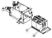
Slide out the battery tray (A) with the batteries.
