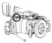
Remove the side-mounted legrests if fitted. A center-mounted, manually adjustable legrest should be either put in its top position by turning the spindle (A) or removed.
