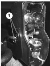
Loosen and remove two screws which hold front headlight.
