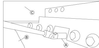
Loosen and remove screw 8 over mud guard 8 under seat frame  $\textcircled{\circ}$ .
