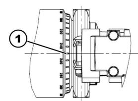
Use scale to align motor to center axis (1), 2-pole motors and 4-pole motors:
