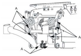
Fix cable with cable ties at locations marked (A).
