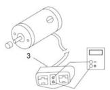
Pull motor plug (3) out of power module.
