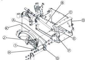
Rotate top walking beam E until Allen screw E is in line with opening D in battery case D.
