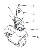
If necessary, remove screw (1) and cap (2).
