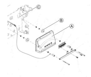
Remove module (a) carefully by lifting rubber stoppers (b) from opening (c).
