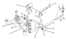
1. Position complete rear wheel suspension between two mounting points (6).
