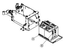
Slide out the battery tray (A) with the batteries.
