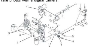
Remove all cables and cable ties which are fixed to wheel suspension or which could get in the way during work.
