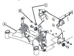
Insert two screws ® together with washers ©.
