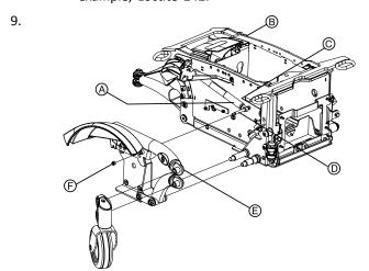
Rotate top walking beam E so that you can reach the screw D on the gas cylinder through the drillhole C in battery box.
