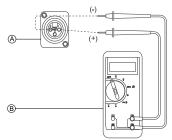
Connect the voltmeter leads to the charger connector (A) on the mobility device. Most digital voltmeters (B) are not affected by polarity. However, analog meters (meters with swinging needles) can be and should be used carefully.
