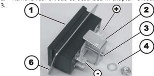
Loosen and remove nut (5) including locking washer (4) using 10 mm socket wrench.
