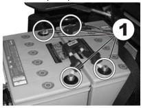
Remove the terminal cover from the battery terminals (1).
