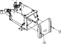
Remove the thumb screws securing the front shroud/battery retention bracket to the wheelchair  ${\bf A}$ .
