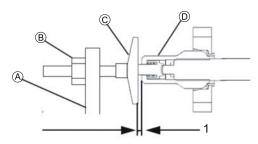
Rotate setting screw © until there is a space of 2 mm (1) between it and the gas cylinder D.
