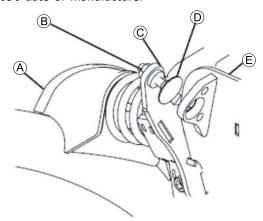
Loosen two screws  ${}^{\circledR}$  and remove together with washers  ${}^{\circledR}$
