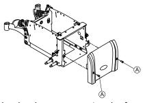
Remove the thumb screws securing the front shroud/battery retention bracket to the wheelchair (A).
