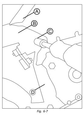
Remove nut  $\mathbb C$  on upper beam  $\mathbb B$ ,  $\mathbb D$  on mud guard  $\mathbb A$ . Hold screw in place.
