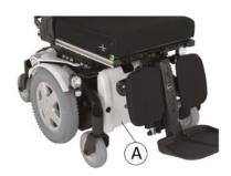
Batteries behind front shroud  $\triangle$  Fig. 6-1
