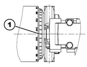
Use scale to align motor to center axis (1), 2-pole motors and 4-pole motors:
