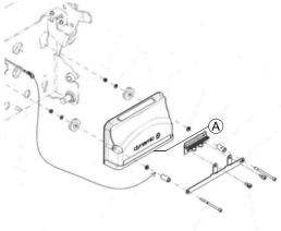
Carefully note location of cable and connection locations of various plugs on power module (a). Either mark each plug and socket, or take a photograph with a digital camera
