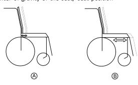
Seat depth  ${}^{\textcircled{}}$  can be adjusted by moving backrest in relation to seat surface.
