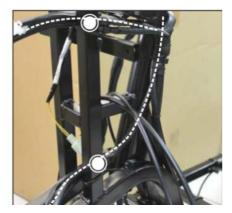
6. Cut the main trace strap on the left side of the front frame (x 2pcs).
