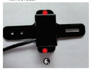
10. The gyroscope can be removed. Please refer backward for reassembly and replacement.
