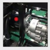
The abnormal sound of the scooter motor during running may be related to the motor/differential mechanism. Please check it first.
