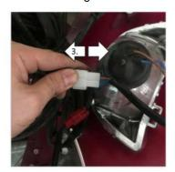
Remove the front slanting screws (M4 x 12L x 1pcs).
