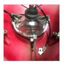
Remove the headlights from the slot. Please refer backward for reassembly and replacement.
