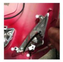
5. Take out the front (left) turn light from the slot. The disassembly method of the left/right turn light is the same.
