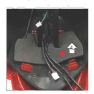
5. Remove the fixing screws of the front shroud and the frame (M4 x 12L x 3pcs).
