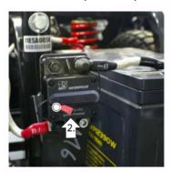
3. After the circuit breaker is pushed up, the reset is completed (as shown below).
