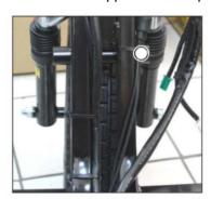
6. The brake trace goes separately from the sides of the frame to connect the left/right rear wheel brake disks. Cut the upper fixed strap (x 4pcs).
