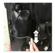
4. Remove the main power switch set from the slot.
