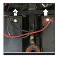
The battery can be removed. 6. Please refer backward for reassembly and replacement.
