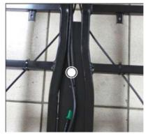
8. The main line extends to the top of the rear frame and cuts the strap (x 1pcs).
