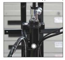
5. Find the relevant connector on the front of the frame. Cut the straps (2 pcs).
