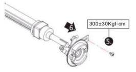
The left/right brake plate can be disassembled in the same way.
