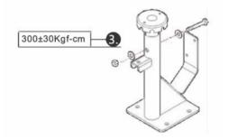
4. The entire set of seat rotating disk can be removed.
