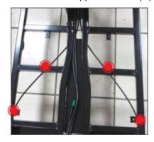
7. Loosen the left/right brake adjustment screws.
