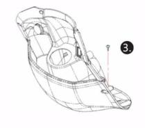
Remove the two screws from the compartment (M4 x12L x2pcs).
