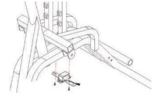
8. The gyroscope set can be removed. Please refer backward for reassembly and replacement.
