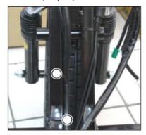
7. The main line passes through the groove at the bottom of the frame. Please directly pull it away from the groove.
