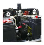
5. Remove the positive and negative terminals on the battery power cable and the battery.
