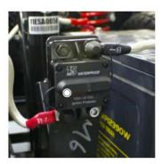
After resetting, switch on to confirm that the scooter is operating normally.
