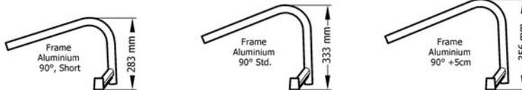
i - (Type of frame in relation to footrest, knee to heel length (UL), front seat height (SHv) and rear wheel size)
