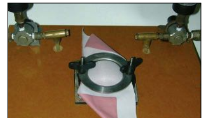
Static head pressure (Porosity testing)
