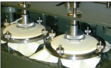
Martindale test (Abrasion testing)
