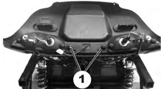
Remove screws (1) on brake light.
