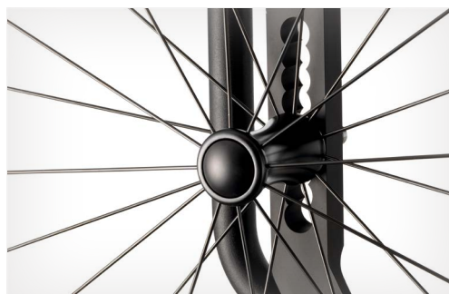
Vertical adapter plate for easy adjustment of the rear wheel position
