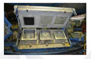
Moulded foams, although more expensive to create and manufacture, can be made with much greater precision. Precise shapes, such as an anatomically formed pelvic well or abductor/adductor contouring, provide better support and fit. Also, the top finish adds durability and is easier to wipe clean compared to cut foam.
