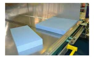
**Slab foam** comes from a foam block that has been cut down to size. In cases where less weight bearing is required, such as in back supports, a single layer of slab foam may provide adequate support and immersion. In cases where more load is applied, such as seat cushions and/or backs used in tilt/recline applications, thicker foam or multiple layers combining softer foam with firmer foam for increased immersion may be used.
