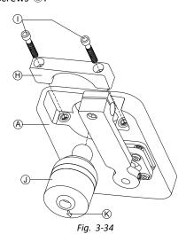
Insert remote ① from below into tray A. Make sure, arrow (shows into reverse driving direction.
