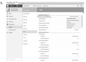
Set **User Input Configuration** to desired component. Options are:
