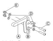
Mount joystick holder A to remote adapter B with screws C , washers D and nuts E.
