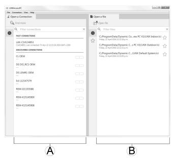
The context modes allow you to work with configuration files both online (that is with a connected system) and offline (that is with files stored on your computer) simultaneously. There are two context modes:
