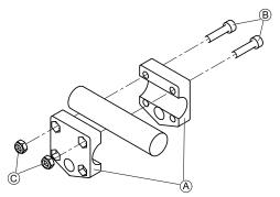
Attach gripper clamp  $\mbox{\textcircled{A}}$  to tube with screws  $\mbox{\textcircled{B}}$  and nuts  $\mbox{\textcircled{C}}.$
