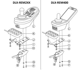
Mount remote 1 to remote adapter 8 and support sheet 1 with screws F and washers G.
