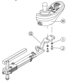
Tighten remote  ${\bf \oplus}$  with screws  ${\bf \oplus}$  and washers  ${\bf \bar{ \top}}$  to bracket  ${\bf @}.$
