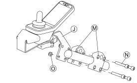
Attach bracket  ${\mathbb J}$  to gripper clamp  ${\mathfrak M}$  with screws  ${\mathbb N}$  and nuts  ${\mathbb O}.$
