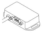
The 4-way button switch or the 4-way toggle switch must be plugged into the DB9 socket.
