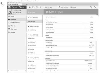
Set Latch Driving in Reverse parameter to On, to allow latched driving in reverse.
