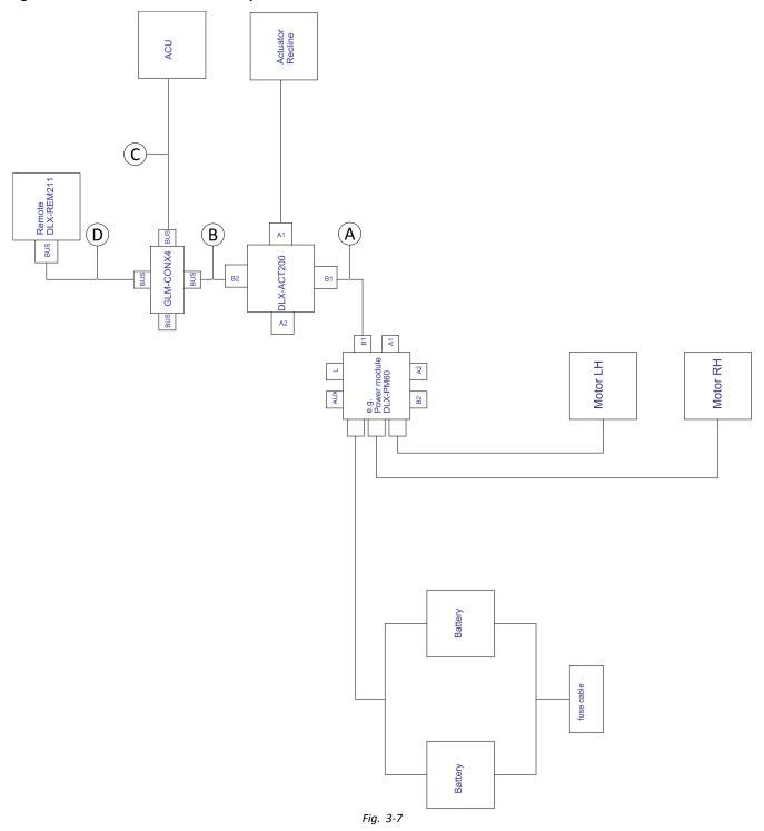
Cable length may vary depending on mounting positions of primary and secondary remotes and of 4–way connector GLM-CONX4.
