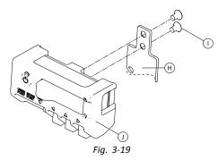
Tighten interface box 1 to holder H with screws 1.
