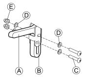
Mount joystick holder A to DLX-CR400 adapter B with screws C, washers D and nuts E.
