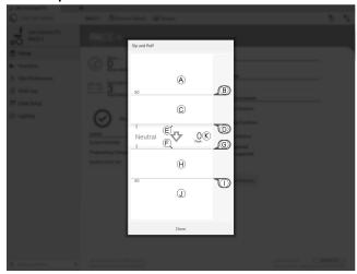
Hard zone for puff input **B** Threshold slider to adjust minimum limit for hard puff Soft zone for puff input Threshold slider to adjust minimum limit for soft puff Neutral zone for puff input Neutral zone for sip input G Threshold slider to adjust minimum limit for soft sip  $\widehat{\mathbf{H}}$ Soft zone for sip input Threshold slider to adjust minimum limit for hard 1 sip Hard zone for sip input
