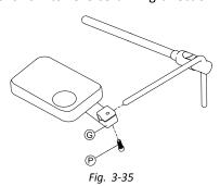
Pull hitch mount © over nucleus and tighten with screw
