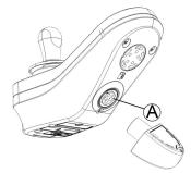
The LiNX Access Key plugs directly into the remote module's XLR port (A). REM2xx displayed in picture, works for REM400 and REM500 the same way.
