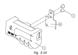
Tighten interface box 1 to holder H with screws 1.
