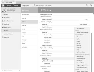
If **Short + Long Press button** is selected, assign desired action to **Short Press** and **Long Press**.
