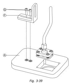
Mount angle bracket (F) with screws (G) to tray (A).
