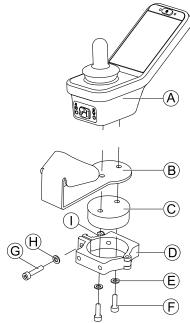
Mount remote A with support B and support drum C to clamp D with screws F and washers E.
