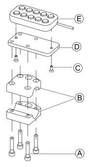
The 10 way switch is fitted to the rear of the wheelchair using a bracket  ${\mathbb B}$  on the push handle or push bar.
