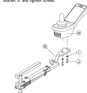
Tighten remote with screws (A) to bracket (G).
