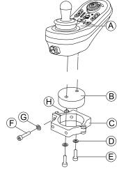
Mount remote A with and support drum B to clamp C with screws E and washers D.
