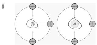
If a gyro module is enabled, the graphic in the center of the graph changes from a person in a wheelchair to a gyroscope to indicate that the parameter being changed are gyro-specific.
