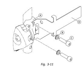
Loosen and remove upper screw © and washer ®.
