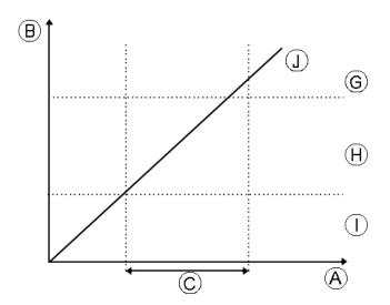
When setting **Sip and Puff Ramp Time**, consideration should be given to users, who cannot produce a hard sip or puff within the ramp time. If ramp time is set too low, a user may not be able to reach the hard zone s in time and a soft sip or puff is registered instead of the intended hard sip or puff. For users who need more time to reach hard zone, the ramp time s needs to be extended, so the pressure input s is registered as a hard sip or puff.
