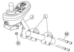
Attach bracket  ${\rm \textcircled{1}}$  to gripper clamp  ${\rm \textcircled{L}}$  with screws  ${\rm \textcircled{M}}$  and nuts  ${\rm \textcircled{N}}.$
