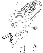
Mount remote  $\theta$  to remote adapter  $\theta$  with screws  $\theta$  and washers  $\theta$
