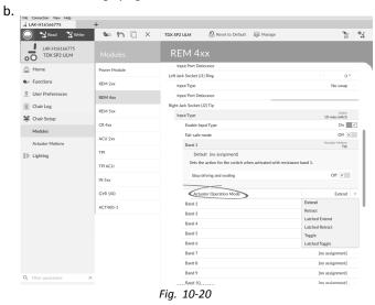
If actuator motion is assigned to parameter, **Actuator Operation Mode** must be selected.
