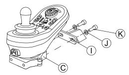
Attach clamp  $\ \textcircled{e}$  to bracket  $\ \textcircled{1}$  with screws  $\ \textcircled{k}$  and washers  $\ \textcircled{1}$  .
