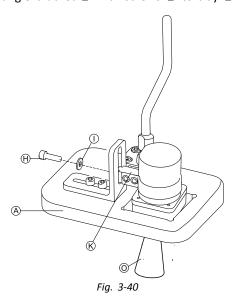
Fix adapter block  $\ensuremath{\mathfrak{C}}$  to angle bracket  $\ensuremath{\mathfrak{F}}$  with screw  $\ensuremath{\mathfrak{H}}$ and washer ①.
