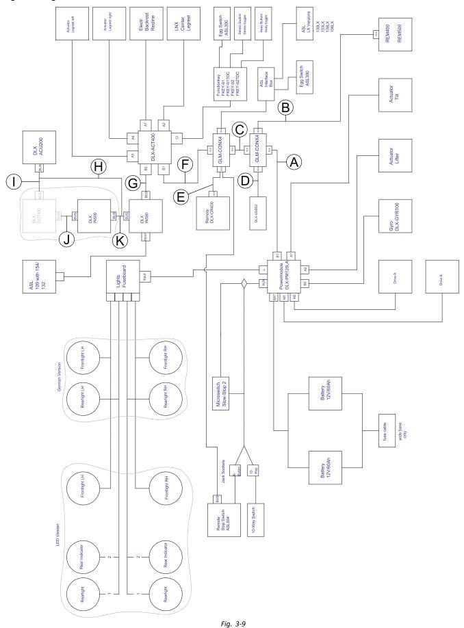
$\frac{\circ}{1}$  Cable length may vary depending on mounting positions of primary and secondary remotes and of 4–way connector GLM-CONX4.
