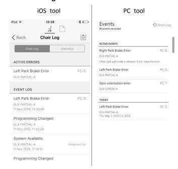
Click on the **Active Errors** button to view which errors, if any, are current. Each entry in this log displays the error, its flash code (e.g. FC5) and the component where the error is. Click on the error entry to reveal an error description with more helpful information about the error.
