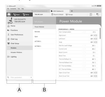
The secondary navigation bar ® is only displayed for certain primary navigation bar selections ® and provides a means to drill down further through the features, functions and parameters.
