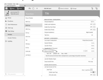
Use this parameter to reduce the effect of hand tremors on the joystick. Low values are suitable for users with low frequency (slow) tremors. Higher values will suit users with higher frequency (fast) tremors. Setting the parameter value to 0 % results in no tremor dampening.
