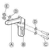
Mount joystick holder A to remote adapter B with screws C , washers D and nuts E.
