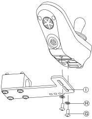
Fix remote to bracket  $\odot$  with screws  $\bigcirc$  and washers  $\bigcirc$  .
