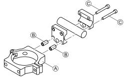
Attach clamp ( ) and spacers ( ) to gripper clamp with screws ( ).
