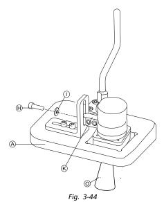
Fix adapter block  ${\mathfrak M}$  to angle bracket  ${\mathfrak H}$  with screw  ${\mathbb J}$  and washer  ${\mathfrak K}$ .
