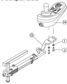
Tighten remote  $\oplus$  with screws  $\oplus$  and washers  $\ensuremath{\ensuremath{\mathbb{T}}}$  to bracket  $\ensuremath{\ensuremath{\mathbb{G}}}.$
