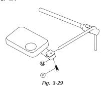
Pull hitch mount © over nucleus and tighten with screw
