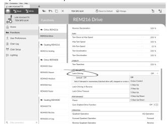
Set type of latched driving with **Latch Driving**. For more information about types of latched driving, refer to user manual of remote.
