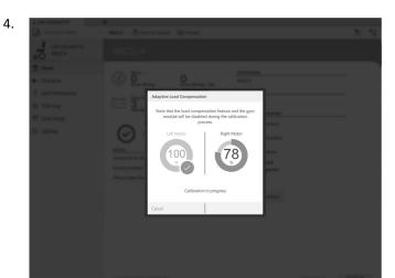
Drive chair until both left and right motor compensation processes have been completed.
