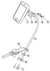
Insert bracket  $\odot$  into joint arm  $\mathbb{B}$ , clamp ball  $\mathbb{N}$  and clamp ring  $\mathbb{M}$ .
