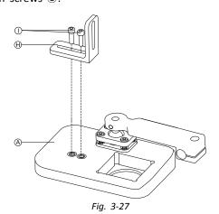
Mount angle bracket  $\oplus$  with screws  $\odot$  to tray A.
