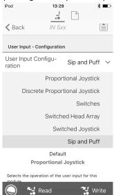
Set **User Input Configuration** to desired component. Options are:
