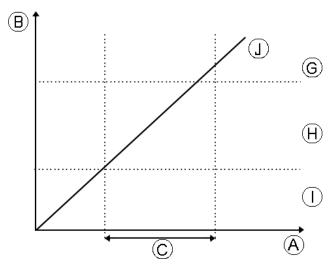
When setting **Sip and Puff Ramp Time**, consideration should be given to users, who cannot produce a hard sip or puff within the ramp time. If ramp time is set too low, a user may not be able to reach the hard zone s in time and a soft sip or puff is registered instead of the intended hard sip or puff. For users who need more time to reach hard zone, the ramp time s needs to be extended, so the pressure input s is registered as a hard sip or puff.
