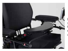
Driving the wheelchair with these switches means that the driver simply needs to cover the sensor corresponding to the desired function: forward, left, right. The fourth switch can be used for reverse or to change function. Drivers can activate multiple switches at the same time.
