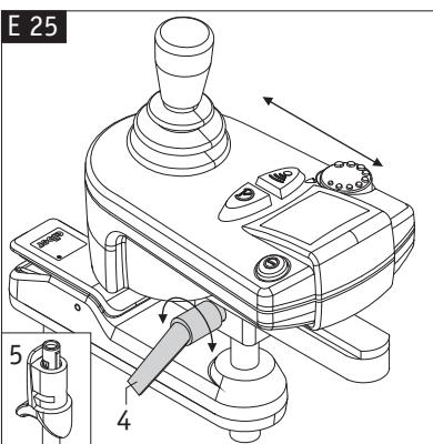
**!** Always switch off the control unit prior to attachment or removal! This prevents your wheelchair from rolling away unintentionally, e.g. due to accidental contact with the joystick.
