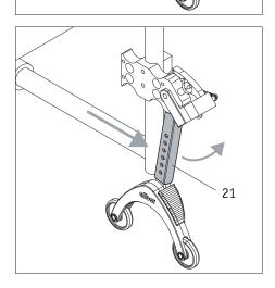
• Once the wheels are fitted, you can return the anti-tippers to their starting position. To do this, push the wheelchair forwards and push back the holding rod [21] using your foot at the same time.
