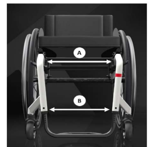
Standard A = SB - 64 mm B = SB - 110 mm (Rahmen kurz) SB - 120 mm (Rahmen Standard) SB - 124 mm (Rahmen + 50 mm)
