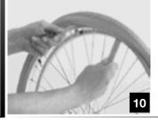
▲ Pneumatic tyres wear out. In addition, the roughness of the ground surface and driving have an impact on their longevity. Replace them regularly to avoid trouble caused by puncture. Please consult with your Dealer.
