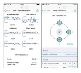
Professionals can now configure powerchairs quickly and more intuitively to each individual user thanks to the revolutionary programming interface built into LiNX.
