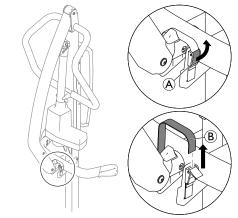
Open the fastener A and remove the band B from the clamping buckle.
