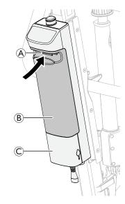
2. Lift the battery up and out away from the Control Unit © or Charger Base ©.
