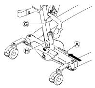
Reinstall the locking pin A through the mast G and base H. Ensure that the locking pin is correctly inserted.
