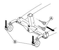
Lock both rear castors  ${}^{\circledR}$  and rotate the hand screws anti-clockwise  ${}^{\circledR}$  to remove them from the base
