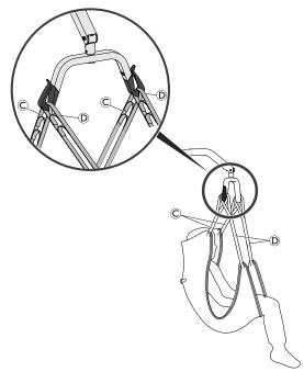
b. On a 4-point spreader bar, attach each of the straps to an individual hook.
