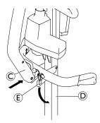
Push and hold the boom  $\mathbb C$  towards the mast  $\mathbb D$  and fold down the spreader bar holder  $\bar{\mathbb E}.$
