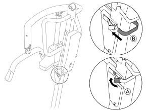
Wrap the band  ${\mathbb B}$  around the back of the mast, insert it into the clamping buckle and close the fastener  ${\mathbb A}$ .
