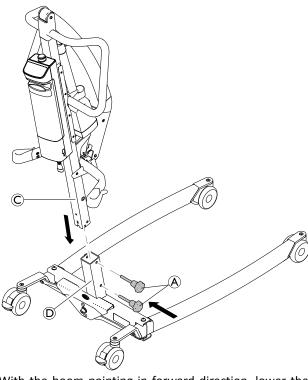
With the boom pointing in forward direction, lower the mast  $\bigcirc$  into the support of base  $\bigcirc$  and reinstall the hand screws  $\bigcirc$  to fix the mast  $\bigcirc$  to the base.
