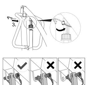
Align the holes and reinstall the pin (a). Make sure that the pin is completely inserted and secure it with the D-clip.
