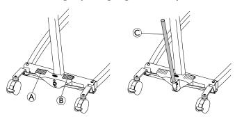
The manual leg spreader is operated by two pedals (A and B) or by the lever C.
