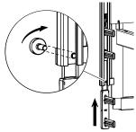
Loosen the screw at the bottom of the guides on one of the bed ends and push the glider halfway up into the guide until it attaches with an audible click.
