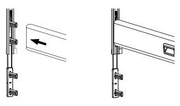
Push the upper side rail onto the two upper pawls.
