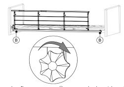
Tighten the finger screws ® to attach the side rail on the top frame. Make sure it is steady and fastened.
