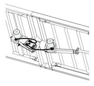
4. Guide the mains cable through the motor pipe pin and the frame hook on the side of the bed that's closer to the power outlet.
