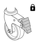
Locking the brake - Step on the outer part  $\ensuremath{\mathbb{B}}$  of the brake pedal
