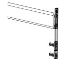
In the other end of the side rail bar; push the two upper pawls into the end of the bar.
