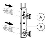
Push the pawl (A) from the backside, through the glider (B) and make sure it locks with an audible click.
