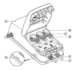
The control box  ${}^{\mbox{$\triangle$}}$  is provided with a label with symbols showing where to connect the motor plugs:
