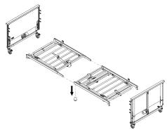
2. Push the inserts on the upper half of the mattress support into the side tubes on the lower half of the mattress support.
