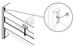
Press the gliding system latch A on one end of the bed and lower the side rail to the lowest position.
