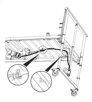
8. Make sure the pipe pins are properly locked.
