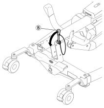
Rotate the locking pin  ${}^{\circledR}$  anti-clockwise to unlock the pivot pin  ${}^{\circledR}$  .
