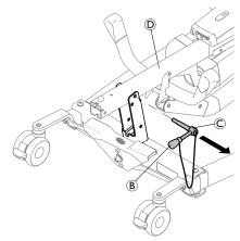
Hold the mast-boom assembly D in position and remove the pivot pin C with the locking pin B.
