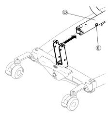
Remove the mast-boom assembly
