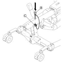
Insert the locking pin  $\ensuremath{\mathbb{B}}$  into the hole on the pivot pin  $\ensuremath{\mathbb{C}}.$
