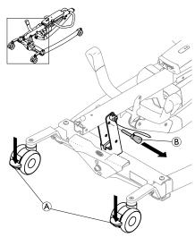
Lock both rear castors A and remove the locking pin B.
