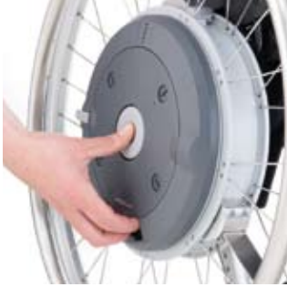
Drive wheels Easy to detach from wheelchair, available in diameters 22" and 24".
