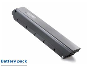
Auto contacting, quick-release battery pack, range up to 50 km (depending on the ground surface, the weight of the user, temperature, wheelchair settings and terrain), weight: only 2.9 kg, battery can be charged in the installed or removed state, optionally available spare battery pack for even more range.
