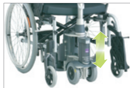
Two wheelchairs in one: the drive wheels are raised electrically.
