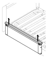
Pull the top bar upwards with both hands near the left and right end.
