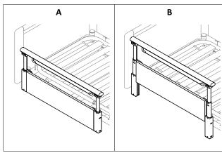
To raise the side rail to the middle position (A), stop pulling upwards after a first audible click. To raise the side rail to the high position (B), pull upwards to the upper stop.
