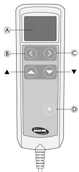
The hand control is equipped with an LCD display A, navigation buttons (B and C) to select the electrical functions and up and down buttons (A and V) to control the selected function.
