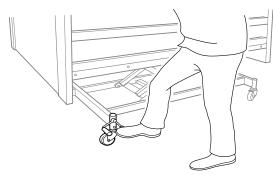
Always stand in the middle of the bed's long side when locking the brakes.
