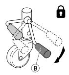
1. Lock the brakes: Step on the red pedal®.
