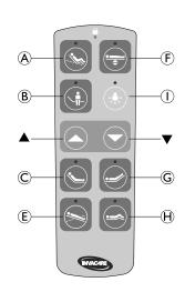
The hand control is equipped with buttons for electrical functions ( $\triangle$  to  $\square$ ), up and down buttons ( $\triangle$  and  $\triangledown$ ) to control the selected function and optionally with a button for an under bed light (①).
