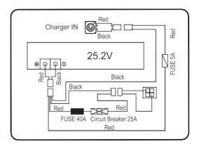
Lead-acid battery - Circuit diagram
