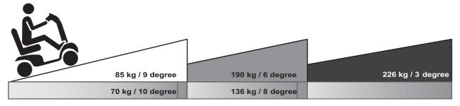
The grade climbing degree will be affected by weight capacity, driving speed, and ramp degree, and scooter parameter. To prevent any danger from a defected motor, please avoid to drive on long ramp or any uneven terrain.
