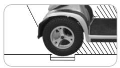
When driving scooter on ramp, adjust body centre of gravity to keep scooter safer.
