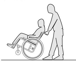
To show the user the tipping point, the wheelchair can be tilted backwards by an assistant using the push bar.
