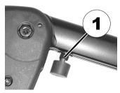
Use the open-ended spanner to loosen the counternut (1).
