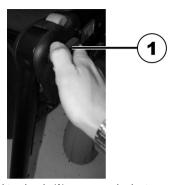
Loosen the locking knob (I) counter-clockwise at least one turn.
