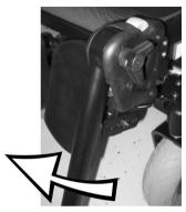
Swivel the legrest upward in order to access the rubber stop.
