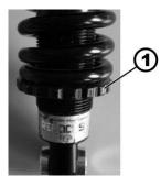
If not, rotate the adjustable spring plate (1) clockwise until the ground clearance is at least 80 mm.
