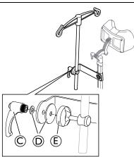
Mount the lever  $\mathbb C$ , the washers  $\mathbb D$  and the holder with the drip stand  $\mathbb E$  in the attachment and tighten the lever.
