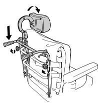
Lower the push handles and tighten the hand wheels.
