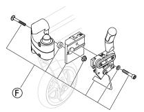
1. Remove and scrap the castor locking and the screws and nuts  $\widehat{\mathbb{F}}.$
