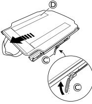
Press the release handle © and push the sliding seat forwards.
