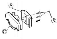
Attach the clamps A with the tilt scale C to the push bar/push handles or the backrest tubes and tighten the screws B.
