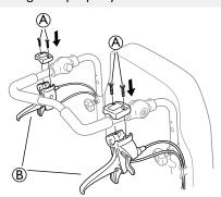
Re-mount the brake handles  $\ensuremath{\mathbb{B}}$  and tighten the screws  $\ensuremath{\mathbb{A}}$ .
