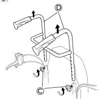
Loosen the handwheels  $\ensuremath{\mathbb{C}}$  and remove the push handles  $\ensuremath{\mathbb{D}}.$
