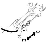
Adjust the tilt resistance with the adjustment nut  ${\bf \hat{A}}$  on the wire.
