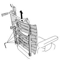
Loosen screws and remove the backrest by lifting upwards.
