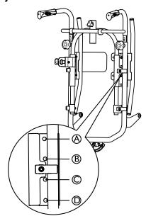
A to D Screws for alternative height adjustment
