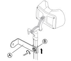
Mount the holder for the drip stand A on the neckrest holder and tighten the screw B.
