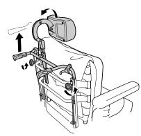
Loosen the handwheels and raise the push handles as far as possible.
