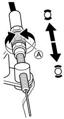
Adjust the brake effect with the adjustment nut  ${\bf \hat{A}}$  on the wire.
