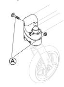
1. Remove and scrap the screw and nut A.
