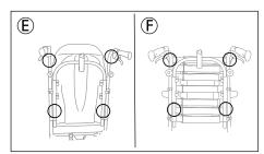
Place the tilt scale for the backrest angle on the push bar/push handle or on the backrest tubes according to picture E or F above.
