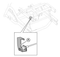
1. Place the holder with the battery cable (A) on the marked area of the frame.
