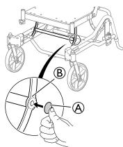
Add the first sealing stickers A over the holes of the cross tube B on both sides.
