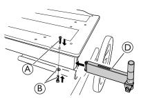
Mount the high legrest attachment ① in the seat frame. Re-insert the upper screw ⓐ and the lower screw and washer ⑧. Re-tighten the screws.
