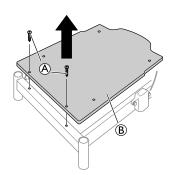
Loosen and remove the screws (A) and the seat plate (B).
