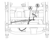
1. Attach the cable for the battery charger (A) and for the battery (B) to the frame with two separate cable ties.
