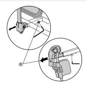
After a period of use, the screws (A) may need to be re-tightened (12Nm).
