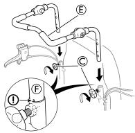
Mount the push bar  $\[ \mathbb{E} \]$  in the backrest tubes and tighten the handwheels  $\[ \mathbb{C} \]$ .
