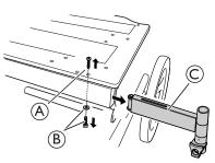
Remove the upper screw (A) and the lower screw and washer (B). Remove the ordinary legrest attachment (C).
