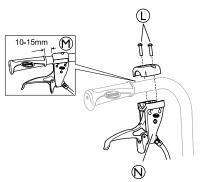
Mount the lever for the assistant maneuvered drum brake  $ext{$\mathbb{A}$}$  on the push handle and attach the screws  $ext{$\mathbb{B}$}$ .
