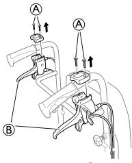
Loosen and remove the screws A and the brake handles B.
