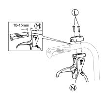
Mount the lever for the assistant maneuvered drum brake  ${\Bbb A}$  on the push handle and attach the screws  ${\Bbb B}$ .
