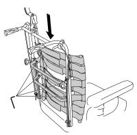
Put the backrest back by fitting it to the receivers on the tubes. Tighten the screws.
