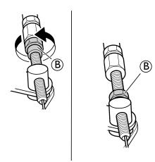
When the desired brake effect is achieved, fixate the brake wire with the fixation nut  $\[ \mathbb{B} \]$ .
