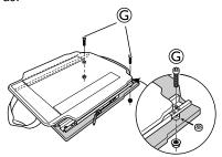
Attach and tighten the rear screws and nuts ©.
