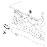
Place the tilt scale for the seat (A) on the seat frame (B).
