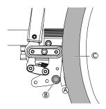
The distance A between the pin B and the tire C should be max. 15 mm.
