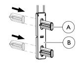
Push the pawl B from the backside, through the glider B and make sure it locks with an audible click.
