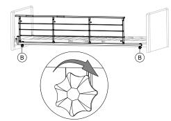
Tighten the finger screws  ${\scriptstyle (\!B\!)}$  to attach the side rail on the top frame. Make sure it is steady and fastened.
