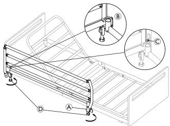
$\begin{tabular}{ll} $\widehat{l}$ & The mounting of the side rail must be done with the side rail in locked position. \end{tabular}$
