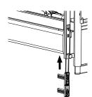
Push the attachment into the guide until it attaches with an audible click (=properly engaged in the lower position).
