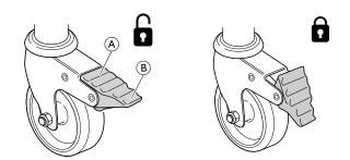
Locking the brake - Step on the outer part  $\ensuremath{\mathbb{B}}$  of the brake pedal
