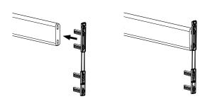
In the other end of the side rail bar; push the two upper pawls into the end of the bar.
