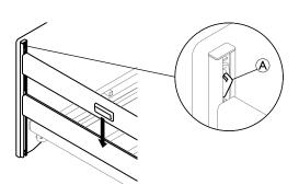
Press the gliding system latch B on one end of the bed and lower the side rail to the lowest position.
