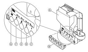
The control box B is provided with a locking cam B and a label with symbols showing where to connect the motor plugs:
