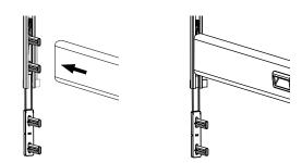
Push the upper side rail onto the two upper pawls.
