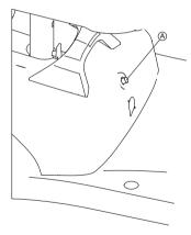
1. To reset, press the circuit breaker button (A) located on the front of the battery box.
