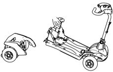
Pull up the seat post to lift up the chassis and hook the chassis onto the drive unit.
