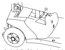
Make sure the latch (A) of the battery box is locked.
