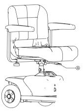
The seat lever A is located under the seat in the front.
