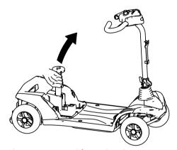
Pull up the seat post to lift up the chassis.
