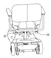
The knobs for releasing the armrests are located under the seat  $\hat{\mathbb{A}}$ .
