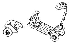
The drive unit separates from the chassis.
