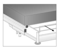
Release the centrally located spring and pull out the mattress support extension.
