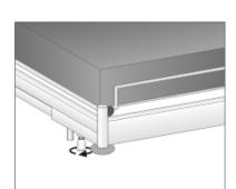
Remove the bed end plate in the foot end and loosen the screws on both sides.
