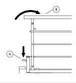
Press the release button B and push the top bar B of the side rail away from the locking mechanism
