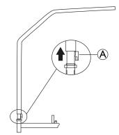
Lift the lifting pole until the control latch (A) is released from the lifting pole tube.
