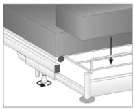
Tighten both screws again and place the extended mattress on the bed.
