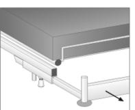
Pull the bed end fitting from the frame. This can be done in two steps of respectively 15 and 20 cm.
