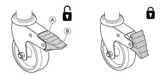
Locking the brake - Step on the outer part  $\ensuremath{\mathbb{B}}$  of the brake pedal
