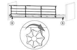
Tighten the finger screws (B) to attach the side rail on the top frame. Make sure it is steady and fastened.
