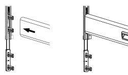
Push the upper side rail onto the two upper pawls.
