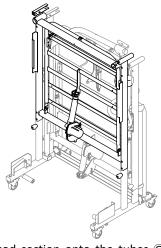
Mount the head section onto the tubes  $\bigcirc$  with the motor facing away from the trolley cross-channel  $\bigcirc$ . Secure the foot section on the trolley with the finger screws.
