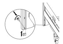
Retighten the screw and tab under the lower side rail bar, in each corner of the bed ends.
