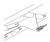
Attach the cable fitting to the hole of the deck bracket with the clevis pin provided and make sure the head of the clevis pin is on the same side as the rastofix deck brackets.
