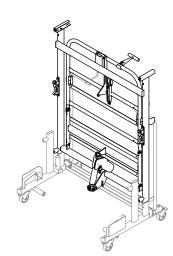
Mount the foot section onto the tubes  $\textcircled{\sc only}$  with the motor facing away from the trolley cross-channel  $\textcircled{\sc only}$ . Secure the foot section on the trolley with the finger screws.
