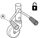
Unlock the brakes: Step on the green pedal
