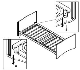
Remove the screws of the bed end brackets on both sides of one bed end.
