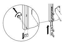
Loosen the screw and tab at the bottom of the guideways on the bed ends and on one side push the glider halfway up into the guideway until it attaches with an audible click.
