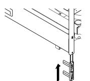
Push the attachment into the guideway until it attaches with an audible click (=properly engaged in the lower position).
