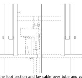
Lift the foot section and lay cable over tube and guide pulley.
