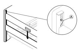
Press the gliding system latch B on one end of the bed and lower the side rail to the lowest position.
