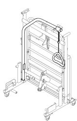
Place the lifting pole onto its location <sup>B</sup>.
