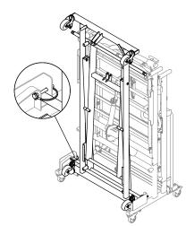
Lift end of base assembly into a vertical position, allowing the square glide bushings to engage into the brackets  $\bigcirc$ . Secure base to trolley with spring pins.
