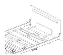
Attach mattress deck extender to the foot end of the mattress deck.
