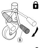
Lock the brakes: Step on the red pedal<sup>®</sup>.
