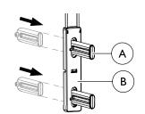
Push the pawl B from the backside, through the glider B and make sure it locks with an audible click.
