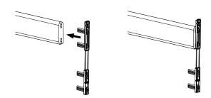
In the other end of the side rail bar, push the two upper pawls into the end of the bar.
