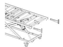
Loosen the screws that secure the standard bed end brackets and remove
