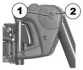
Loosen the screw (1) using the Allen key.
