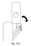
If your mobility device is fitted with a swing-away remote holder, then the remote can be moved away to the side, for example, to drive up close to a table.
