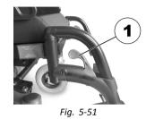
The small release lever is to be found in the upper part of the legrest (1). When the legrest is released it can be swivelled inward or outward to facilitate access and also be removed completely.
