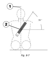
The safety belt installed in the transporting vehicle should be applied as shown in the illustration above.
