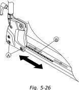
1. Loosen bottom backrest screws (A) on both sides.
