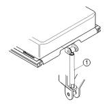
The figure shows the position of the spindle (1) for manual seat angle adjustment.
